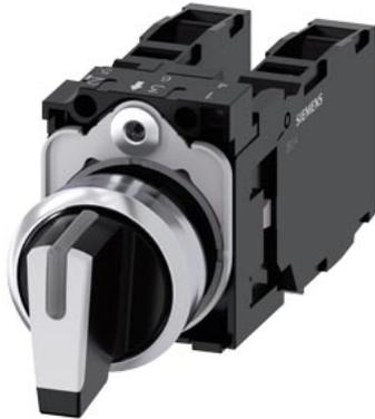
Selector switch, illuminable, 22 mm, round, metal, shiny, white, selector switch, short, 3 switch positions I>O<II, momentary contact type, actuating angle 2x45°, 10:30h/12h/13:30h, with holder, 2x1NO+1NC, screw terminal
