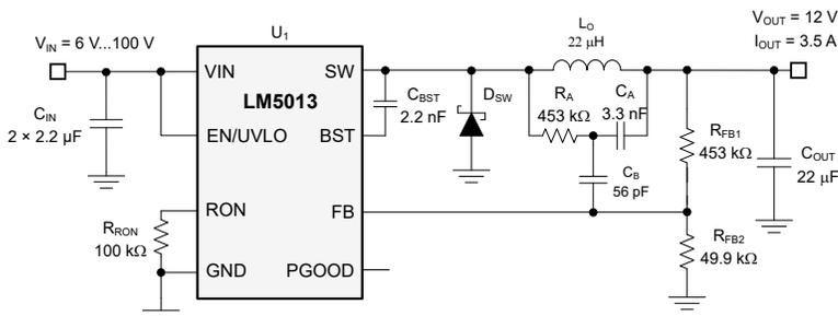
**Typical Application,  $V_{IN(nom)} = 48$  V,  $V_{OUT} = 12$  V,  $I_{OUT(max)} = 3.5$  A,  $f_{SW(nom)} = 300$  kHz**
