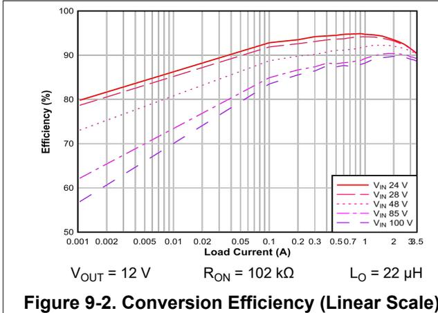
Figure 9-2. Conversion Efficiency (Linear Scale)
