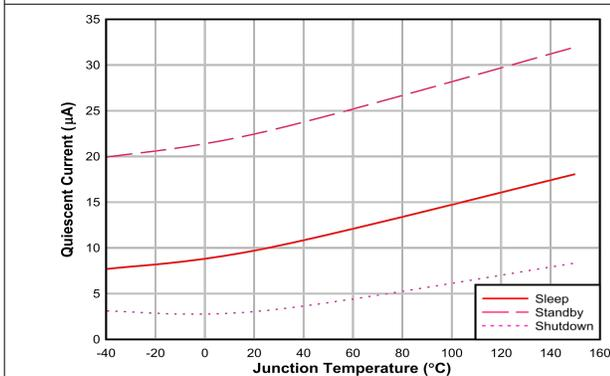
Figure 7-3. Shutdown, Sleep, and Supply Current vs Temperature
