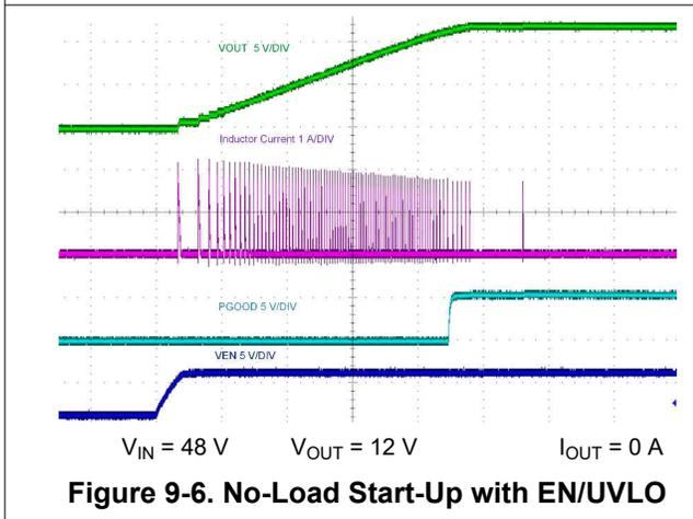
Figure 9-6. No-Load Start-Up with EN/UVLO
