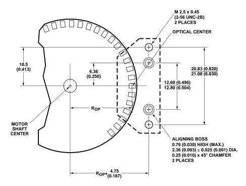
Figure 2. Mounting plane side B.
