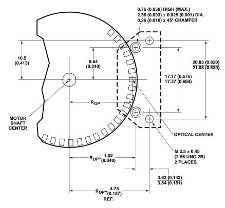
Figure 1. Mounting plane side A.
