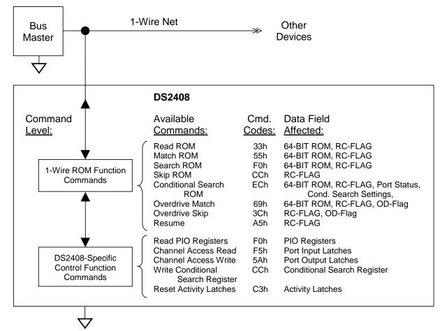
Figure 2. HIERARCHICAL STRUCTURE FOR 1-Wire PROTOCOL
