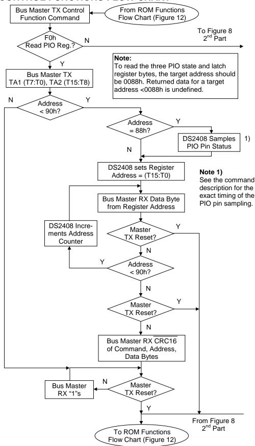
Figure 8-2. CONTROL FUNCTIONS FLOW CHART
