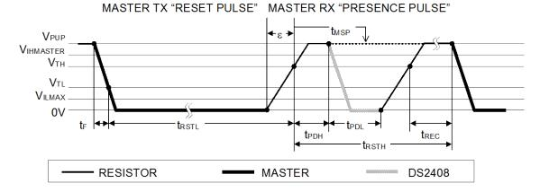
After the bus master has released the line it goes into receive mode (RX). The 1-Wire bus is then pulled to  $V_{PUP}$  via the pullup resistor or, in case of a DS2480B driver, by active circuitry. When the  $V_{TH}$  threshold is crossed, the DS2408 waits for  $t_{PDH}$  and then transmits a Presence Pulse by pulling the line low for  $t_{PDL}$ . To detect a presence pulse, the master must test the logical state of the 1-Wire line at  $t_{MSP}$ .
