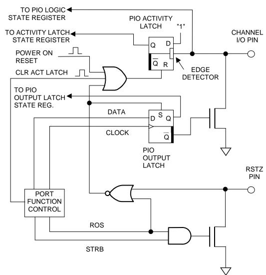
Figure 6. CHANNEL I/O AND RSTZ SIMPLIFIED LOGIC DIAGRAM
