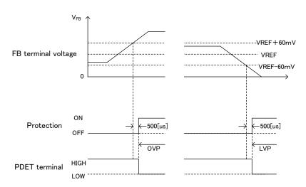
Fig. 5 Output voltage error detection range
