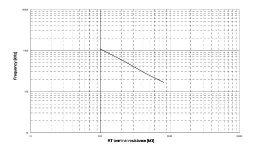
Fig. 4 RT resistance-oscillation frequency
