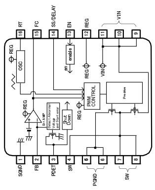
Fig.2 Block diagram
