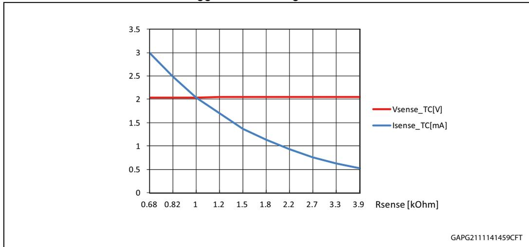
**Figure 97. MultiSense in V<sub>CC</sub> mode behavior versus R<sub>SENSE</sub> for VND7140AJ at V<sub>CC</sub> = 14 V and T<sub>C</sub> = 25 °C**
