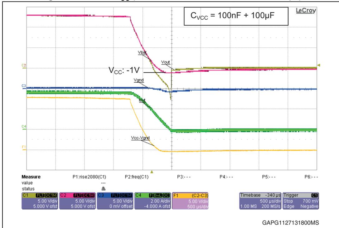
The demagnetization energy (Figure 87) is distributed between the device and  $V_{CC}$  capacitor. The turn-off phase is seen when the  $V_{CC}$  capacitor is discharged below undervoltage. Final voltage on  $V_{CC}$  is  $\sim -1$  V.
