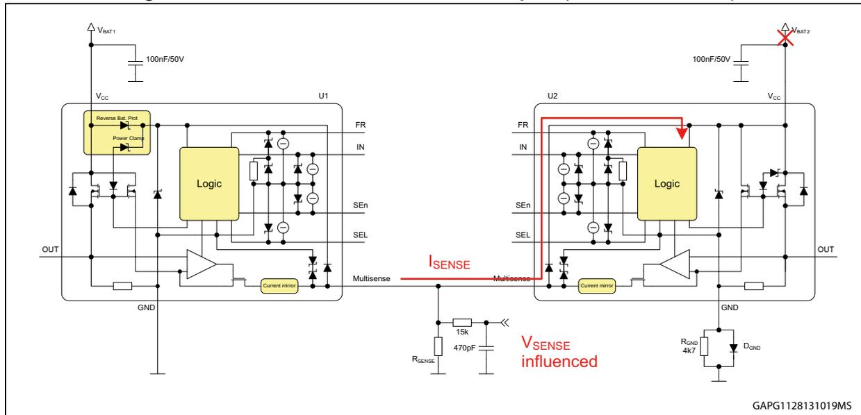
Direct connection of MultiSense pins is not safe in the following cases:
