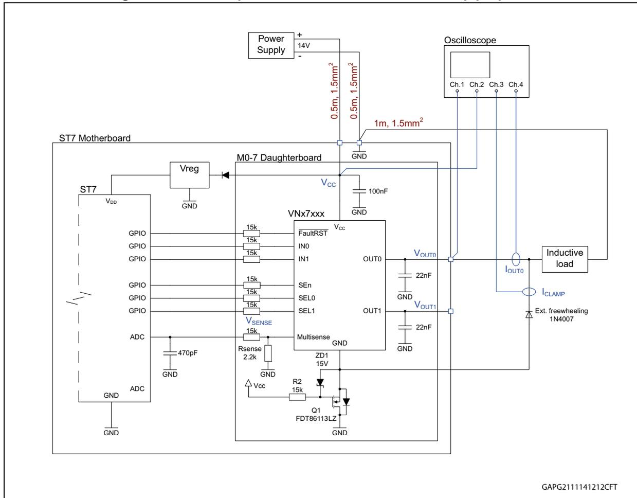
Repetitive operation – PWM 50 % at 100 Hz (the demagnetization time is shorter than the PWM off-state time, see [Figure 79](#)):
