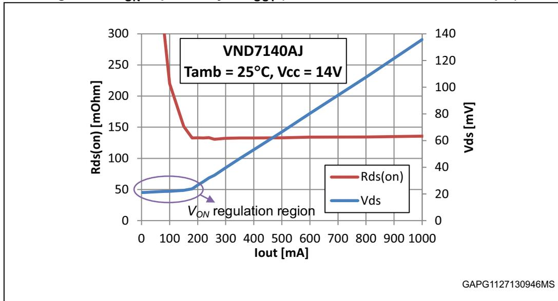
The calculation of conduction losses in PWM mode is based on similar consideration as in case of steady state losses (focusing on R<sub>ON</sub>, I<sub>OUT</sub>, t<sub>on</sub>), however it is important to consider right PWM on time (corrected with the turn-on/off switching delays and switching times) and right current in on state (for instance in case of bulb it depends on actual duty cycle):
