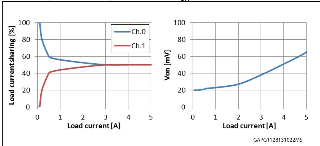
Figure 137. Current sense behavior at low current (VND7020AJ)
