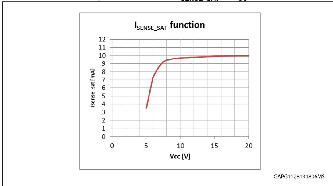
The  $I_{SENSE\_SAT}$  decreases significantly for  $V_{CC}$  below about 10 V. Above this battery level we can consider as minimum value of  $I_{SENSE\_SAT} = 5.2$  V (instead of the minimum of  $I_{SENSE\_SAT} = 4$  mA given in the datasheets at  $V_{CC} = 7$  V). This increases the upper load current range that can be monitored by the current sensing avoiding any saturation
