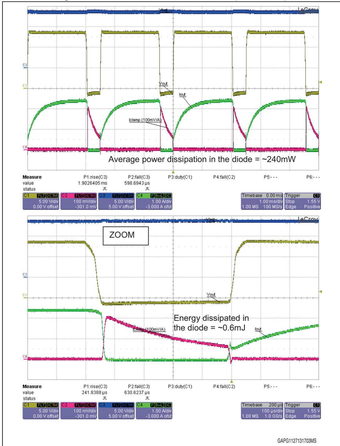
Negative ISO pulse exposure on V<sub>CC</sub> line:
