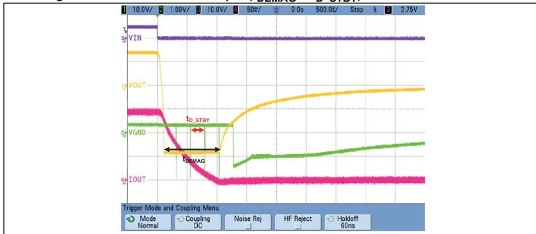
Figure 7. Measurement example ( $t_{DEMAG} > t_{D\_STBY}$ ) with 4.7 kΩ GND resistor
