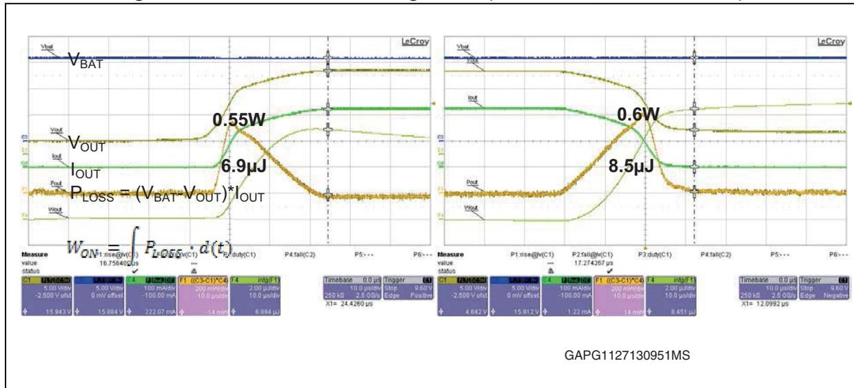
Measured losses: W<sub>ON</sub> ~ 6.9 µJ, W<sub>OFF</sub> ~ 8.5 µJ
