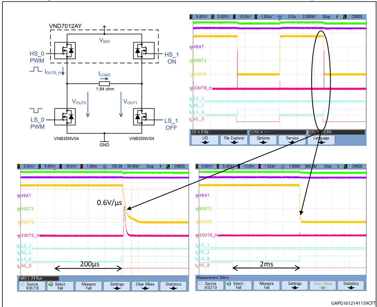
**Cross conduction due to MOSFETs capacitances**
