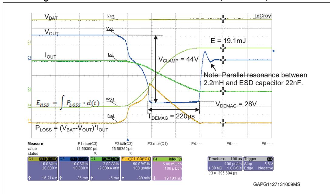
As seen from the oscillogram, measured values are close to the theoretical calculation:  $E_{HSD} = 19.1\text{ mJ}$  (20.1 mJ calculated),  $T_{DEMAG} = 220\text{ } \mu\text{s}$  (235  $\mu\text{s}$  calculated).
