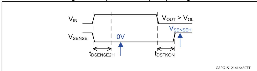
Figure 110. Short circuit to  $V_{BATT}$  timings
