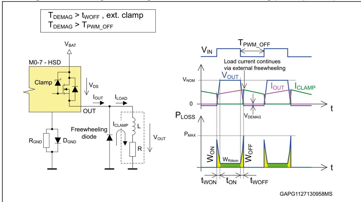
Assuming  $T_{\text{DEMAG}} \gg T_{\text{PWM\_OFF}}$ , the switching losses can be estimated as follows:
