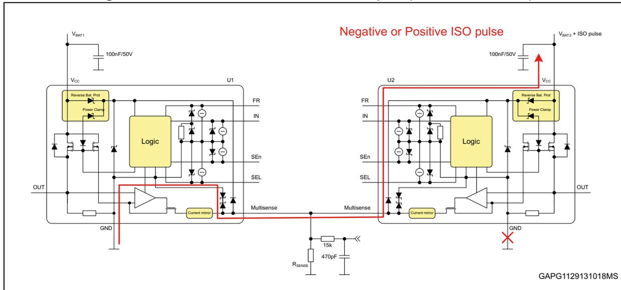
Direct connection of MultiSense pins is not safe in the following case:
