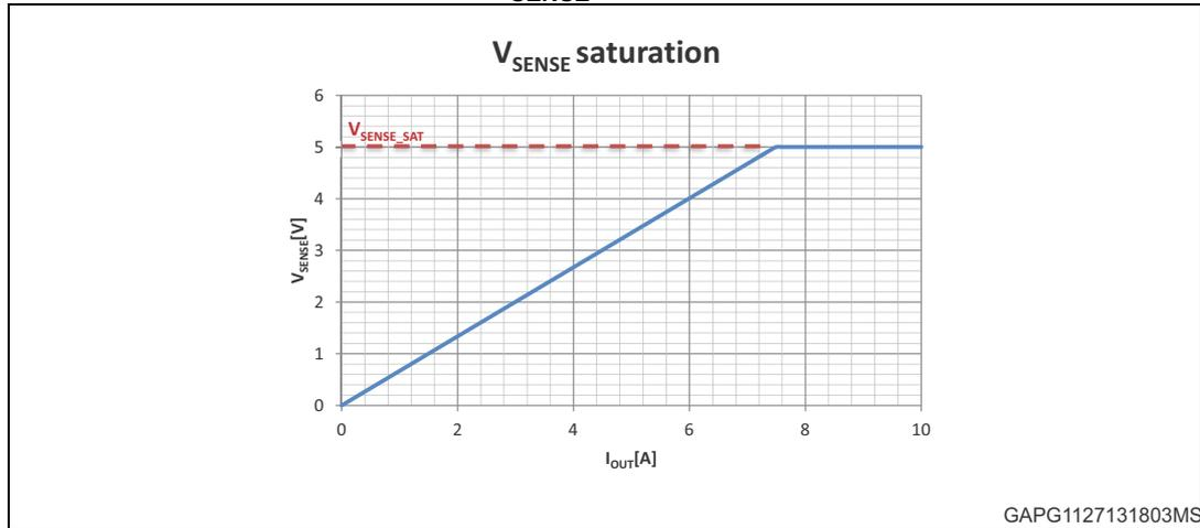
Moreover care must be taken to prevent the current mirror output from saturation, then causing again the  $I_{SENSE}$  no longer to be proportional to  $I_{OUT}$ . This normally happens when the maximum current from the current mirror is reached and corresponds to the minimum value of the parameter  $I_{SENSE\_SAT}$  ( $I_{SENSE\_SAT}$  minimum, reported in the datasheets).
