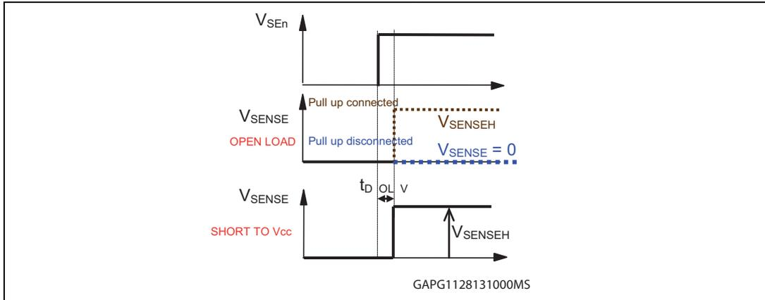
Table 26. MultiSense pin levels in off-state
