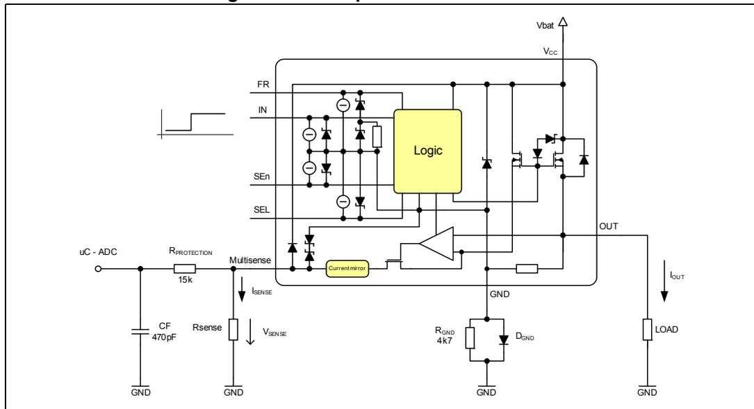
The current sense voltage is usually connected through a 15 kΩ protection resistor to the ADC input of the microcontroller. In case of  $V_{SENSEH}$  level the voltage is limited by the microcontroller internal ESD protection (~5.6 V) while the ADC shows maximum value (0xFF in case of 8-bit resolution). The capacitor CF is used to improve the accuracy of the  $V_{SENSE}$  measurement (refer to [Figure 118](#)).
