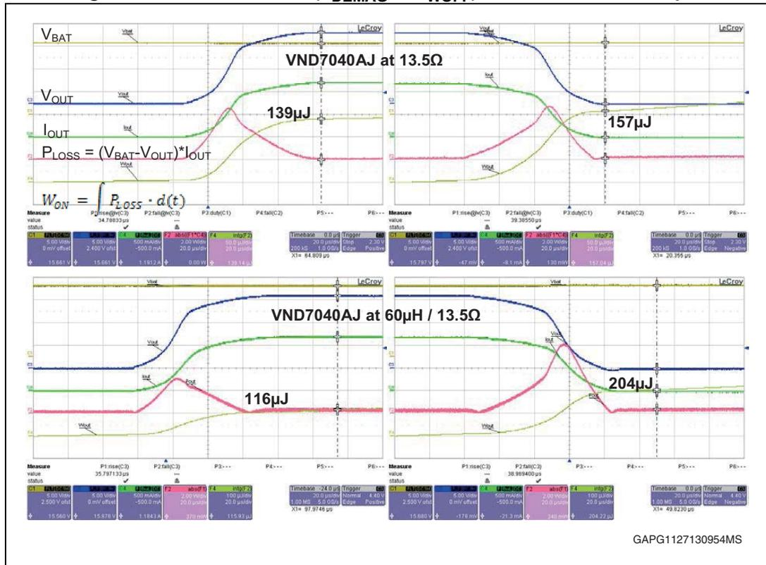
Measured losses (pure resistive 13.5 Ω):  $W_{\text{ON}} \sim 139 \mu\text{J}$ ,  $W_{\text{OFF}} \sim 157 \mu\text{J}$
