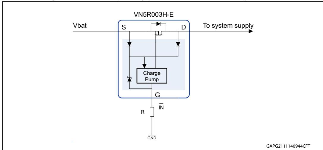
Note that a MOSFET has always an intrinsic anti parallel body diode. If the  $\overline{IN}$  voltage versus drain is negative the device is turned ON. The MOSFET is fully turned on when applying the battery voltage and the  $\overline{IN}$  pin goes negative versus drain. Due to the fact that the Source is at high potential, the MOSFET is a high-side switch not referring to ground; a charge pump circuit is needed to boost the gate voltage over the source voltage to turn the MOSFET on.
