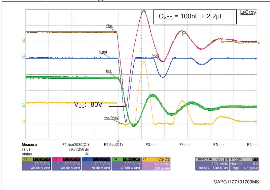
Most of the demagnetization energy (Figure 85) is absorbed by the  $V_{CC}$  capacitor. The voltage peak on the  $V_{CC}$  pin is -80 V. The device channel stays on for the whole demagnetization phase  $\sim 80 \mu$ s. A positive overshoot on  $V_{CC}$  is seen at the end of demagnetization phase, due to the resonance between the  $V_{CC}$  capacitor and load inductance.
