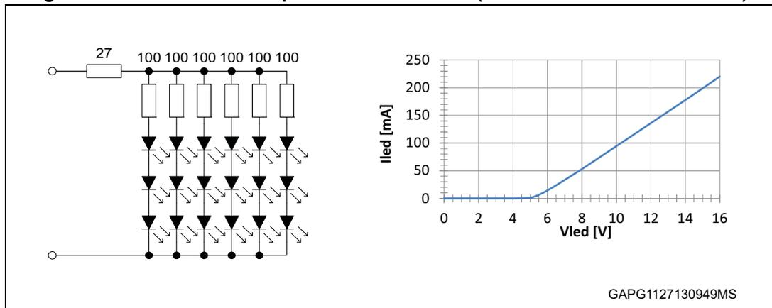
Figure 55. LED cluster example 2–tail & brake light (VW Passat B6)
