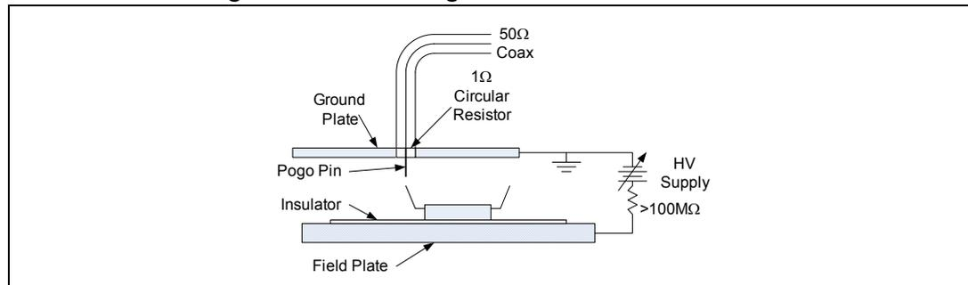
To perform the CDM test an uncharged circuit is placed on the field plate. The field plate is charged to a high voltage and the circuit's potential tracks the field plate. The ground plane is then moved so that the pogo pin touches the integrated circuit, grounding it. The result is
