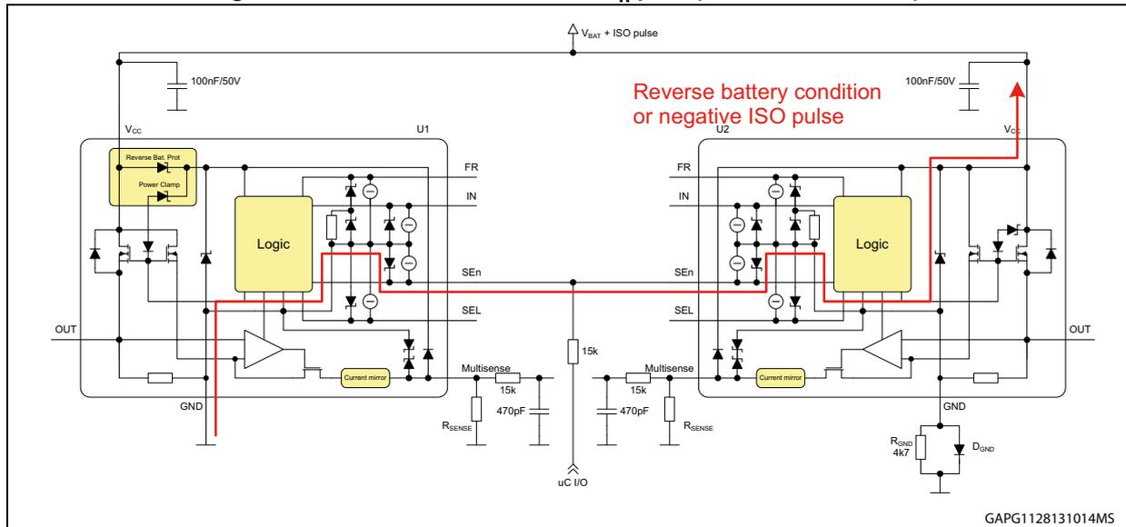
Direct connection of SE<sub>n</sub> pins is not safe in the following cases:
