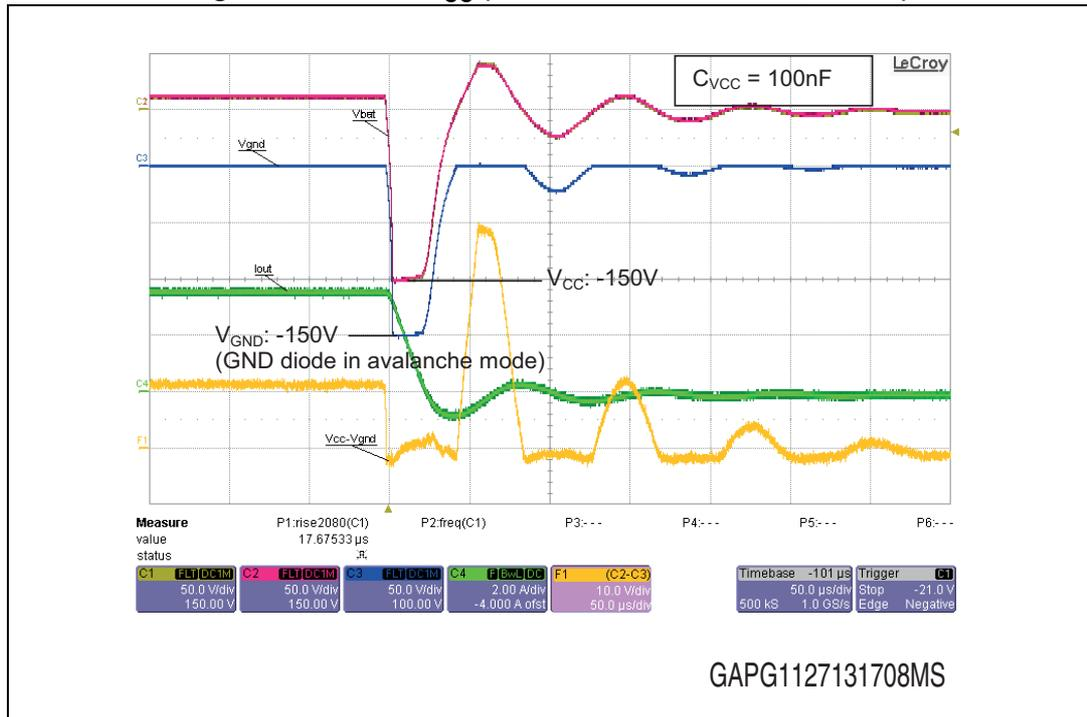
Most of the demagnetization energy (Figure 85) is absorbed by the GND network diode (in avalanche mode). The voltage peak on the  $V_{CC}$  and GND pin is  $\sim 150$  V (equal to break down voltage of the diode). The device channel stays on for whole demagnetization phase  $\sim 30$   $\mu\text{s}$ . A positive overshoot on  $V_{CC}$  is seen at the end of demagnetization phase, due to the resonance between the  $V_{CC}$  capacitor and load inductance.
