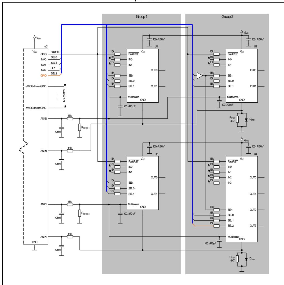
To eliminate the effect of the GND shift variation, it is important to measure the GND voltage and  $V_{CC}$  / Temp signal in the same time (ideally) or with a few  $\mu s$  delay. Possible solutions are shown in the [Figure 122](#).
