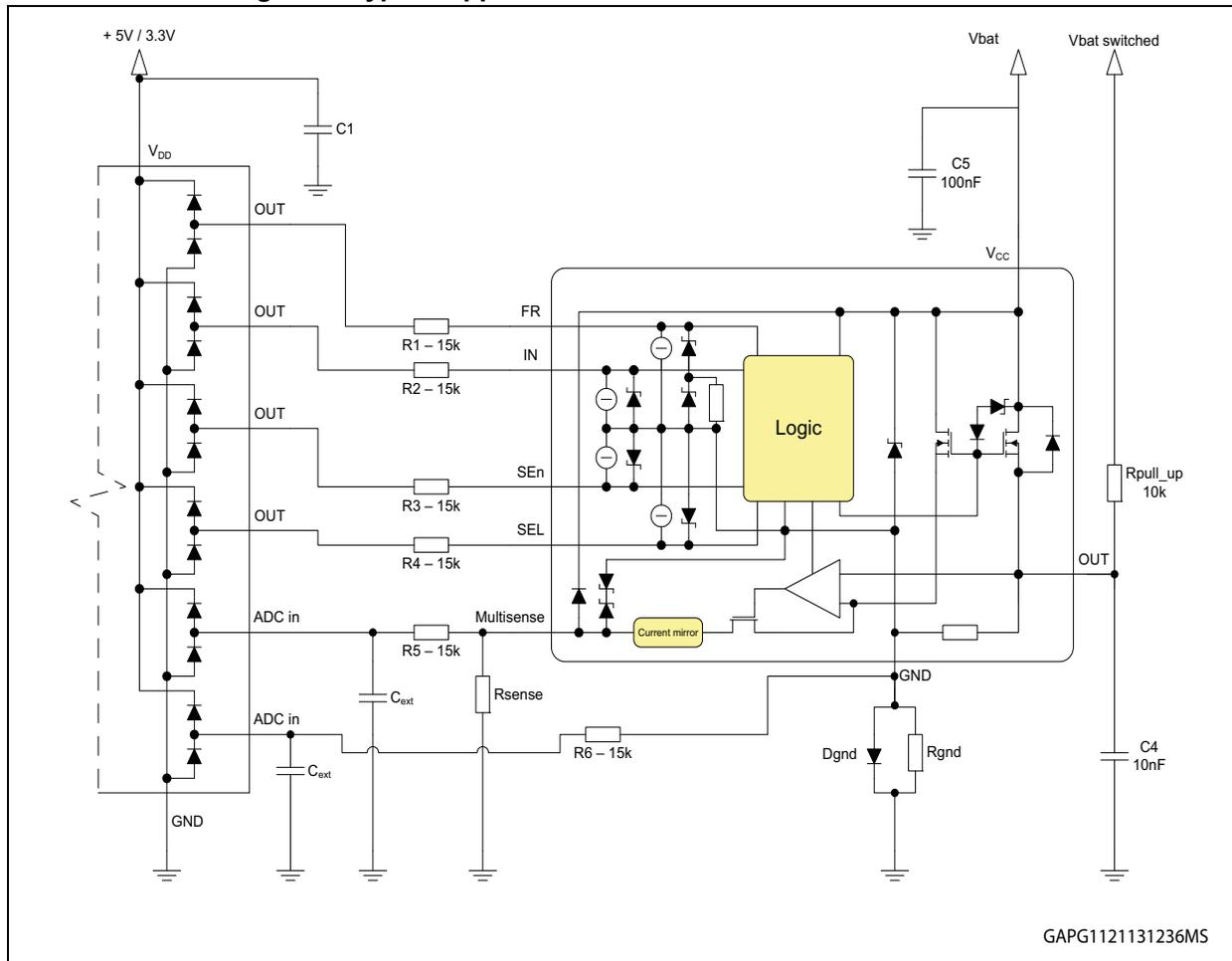
voltage feedback reading is required. For dimensioning the same recommendations apply as for R5//C2.
