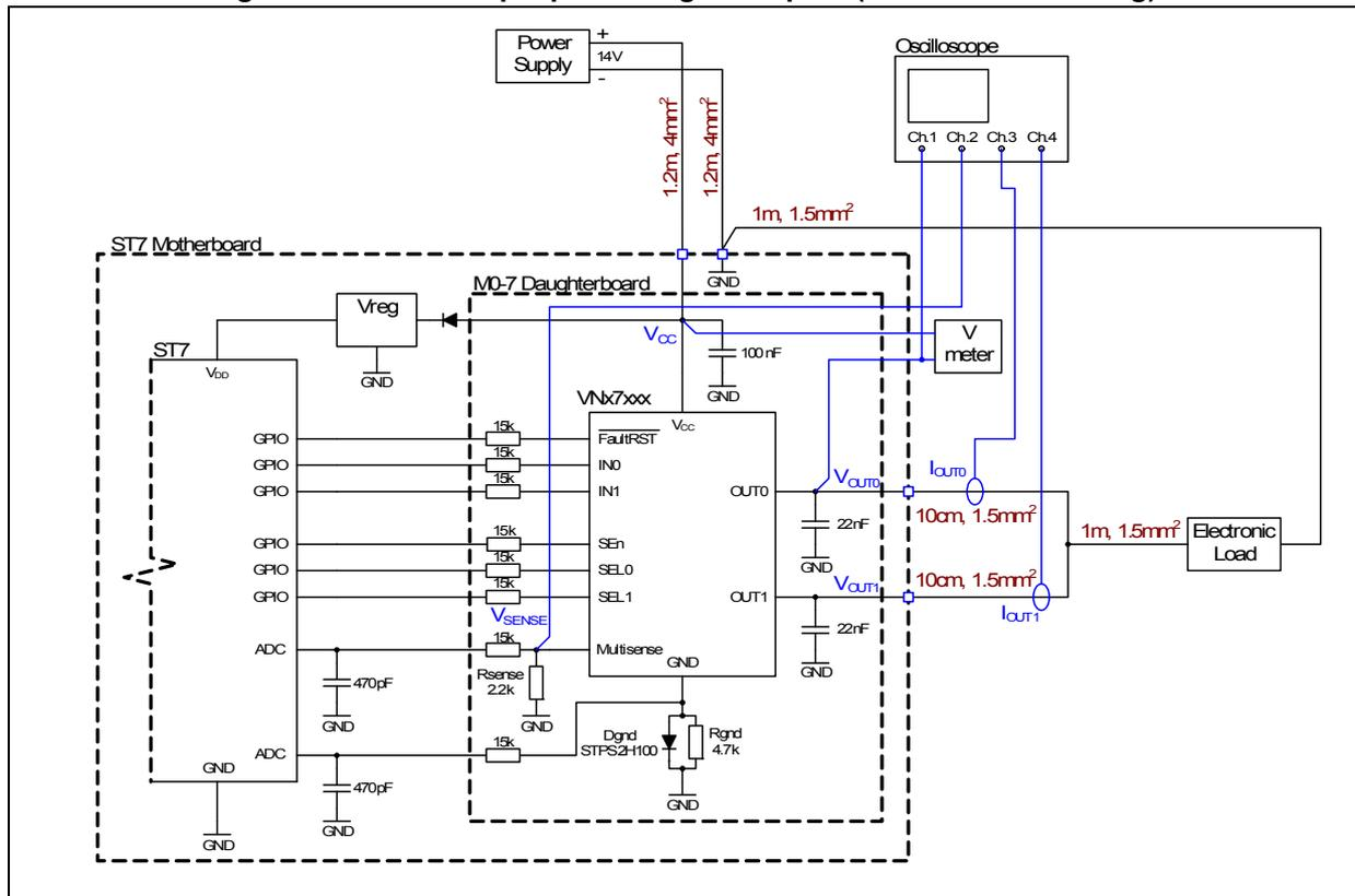
Figure 136. Sharing of load current,  $V_{ON}$  regulation (VND7020AJ)
