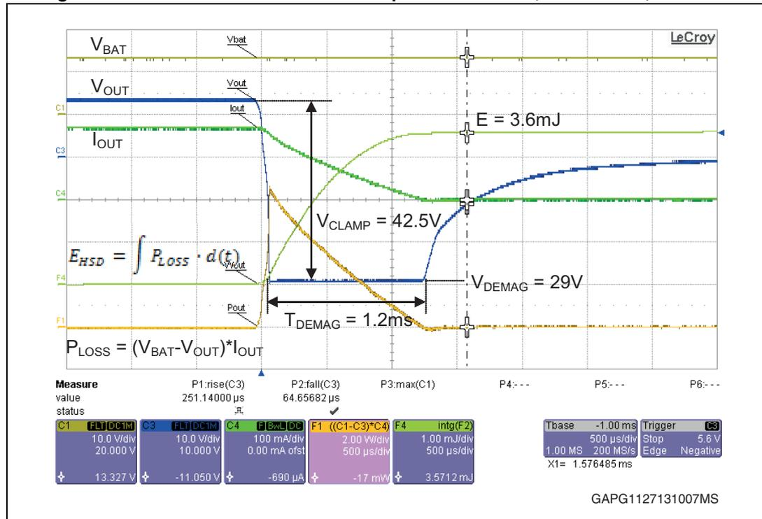
The demagnetization energy dissipated in the HSD was measured by an oscilloscope with mathematical functions. The first function F1 shows the actual power dissipation on the HSD  $(V_{BAT} - V_{OUT}) \cdot I_{OUT}$ , the second function F4 shows the HSD energy (integral of F1).
