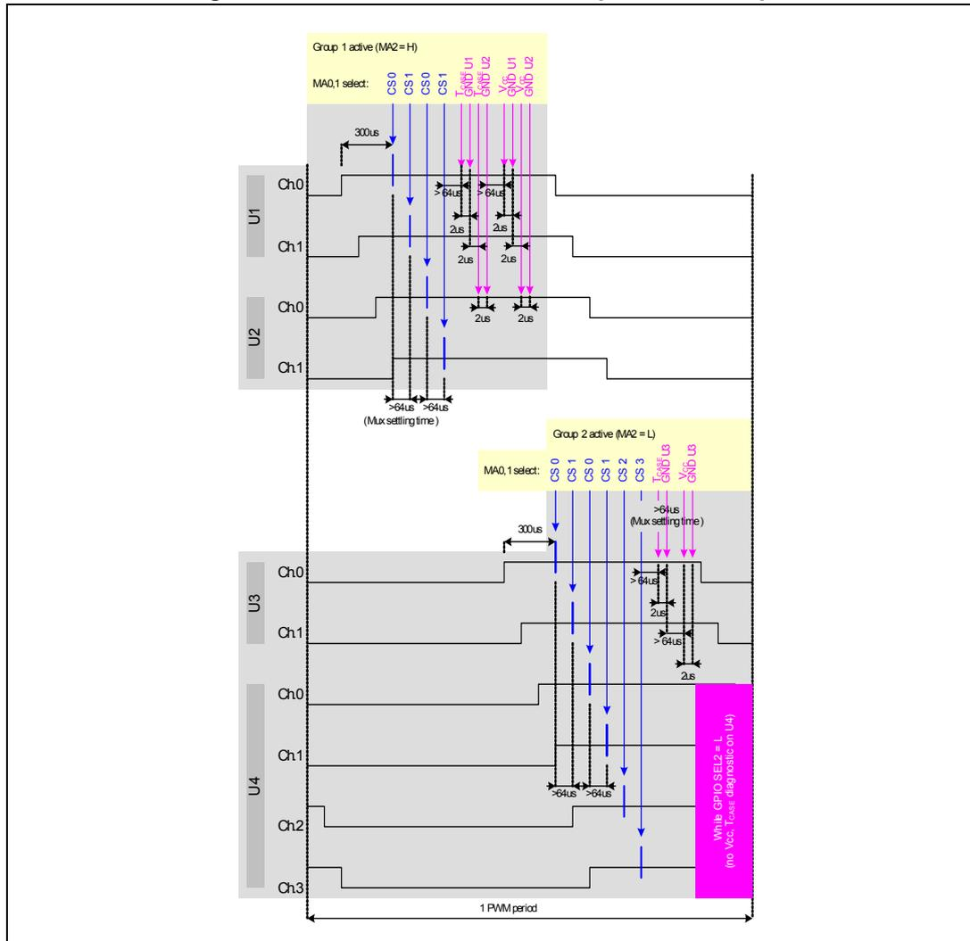
The best trigger position for the  $V_{CC}$ /Temp and the GND voltage measurement is usually after the rising edge of channel with highest phase shift, when all PWM channels are already activated. At that point the GND signal is stable (note that this statement is not valid during power limitation or thermal shutdown).
