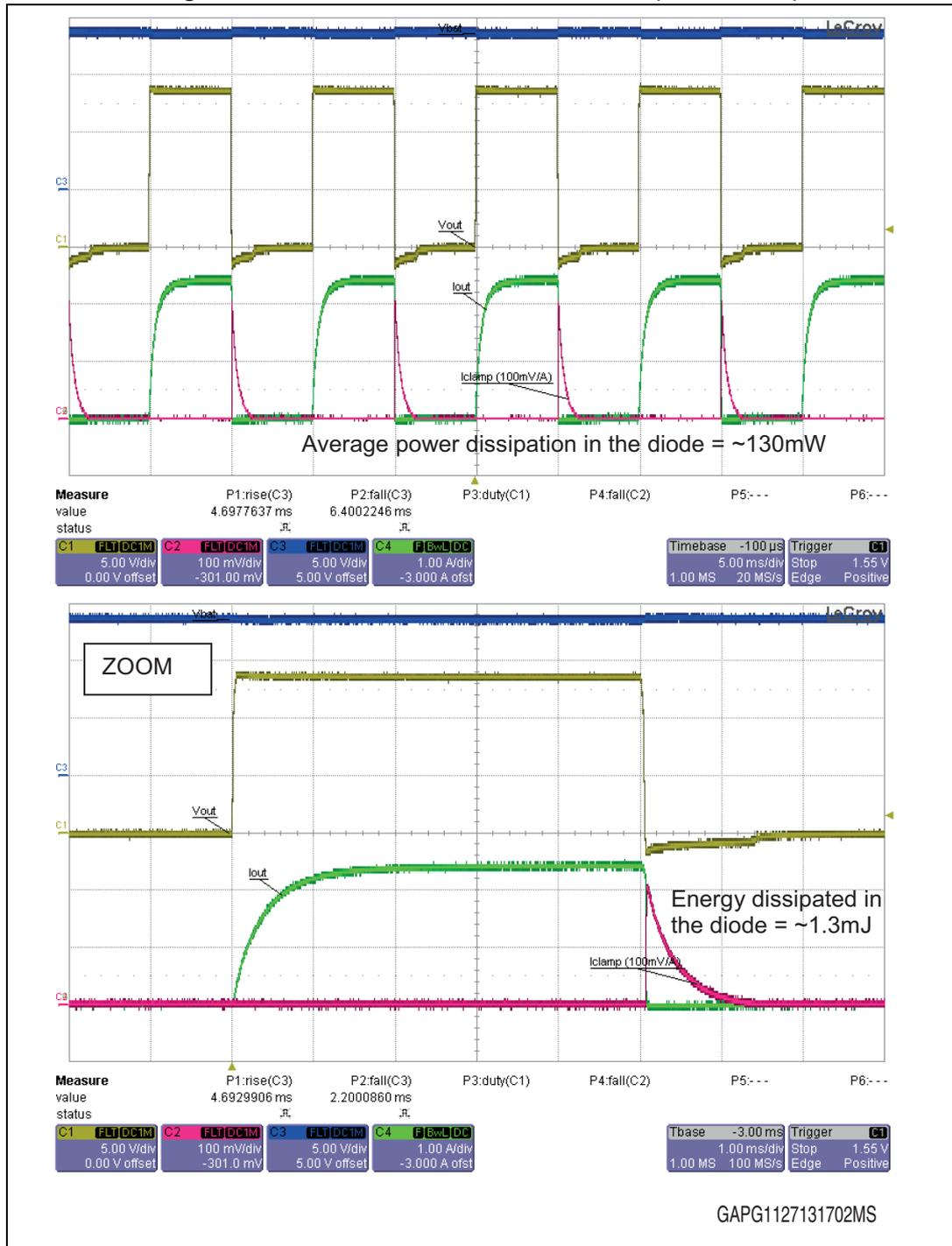
Repetitive operation – PWM 80 % at 400 Hz (the demagnetization time is longer than the PWM off-state time, see [Figure 80](#)):
