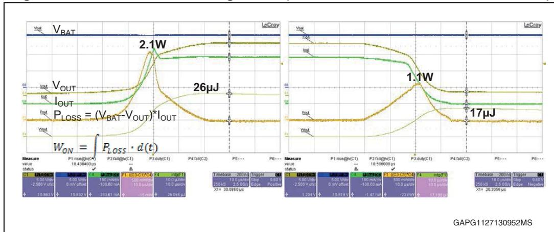
Measured losses:  $W_{ON} \sim 26 \mu\text{J}$ ,  $W_{OFF} \sim 17 \mu\text{J}$
