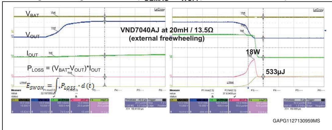
Measured losses (20 mH at 13.5  $\Omega$ ):  $W_{ON} \sim 11 \mu J$ ,  $W_{OFF} \sim 533 \mu J$
