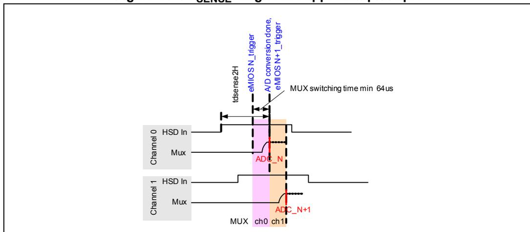
Example configuration applying 0 % CPU load (MUX switching done by microcontroller HW peripherals)
