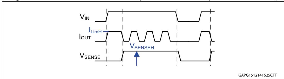
Figure 112. Power limitation or overtemperature waveforms (in latched mode)
