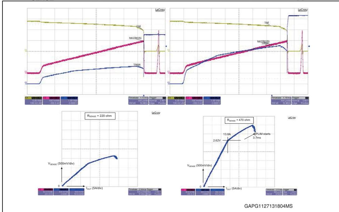
Note:  $V_{SENSE\_SAT}$  and  $I_{SENSE\_SAT}$  minimum values are guaranteed for the minimum  $V_{CC}$  voltage in which all K factor limits are guaranteed (in datasheets this is 7 V) and maximum operating junction temperature (in datasheets this is 150 °C) which represent worst case conditions in the assessment of the maximum load current to be monitored. Experimental Measurements on samples have.
