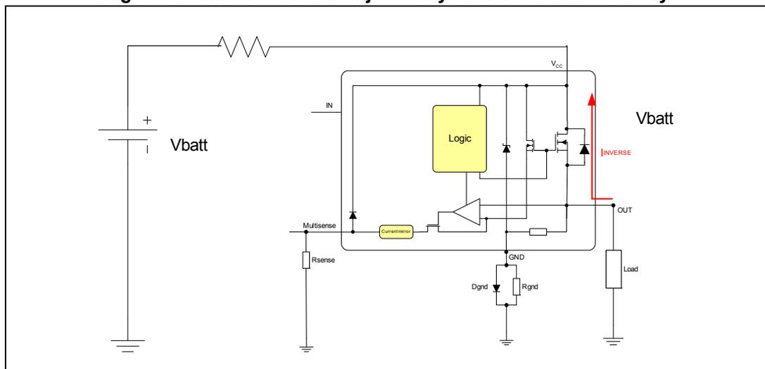
We define  $I_{INVERSE}$  the current that flows into the device from the output.
