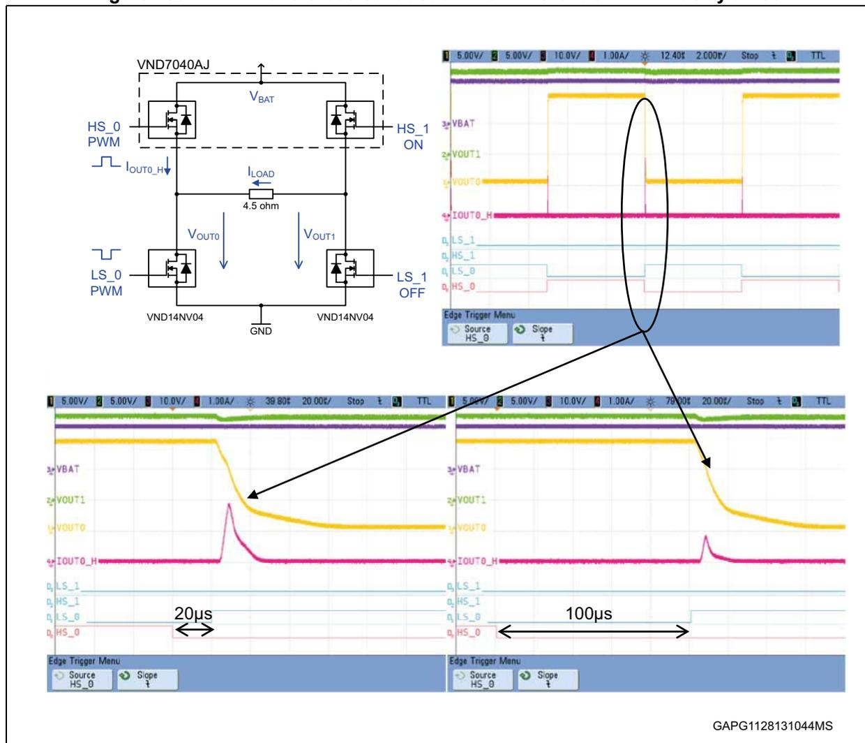
In the left side plot of *Figure 159* a delay of 20 µs only is given, on the right side a delay of 100 µs is given and still it is possible to see a residual cross current.
