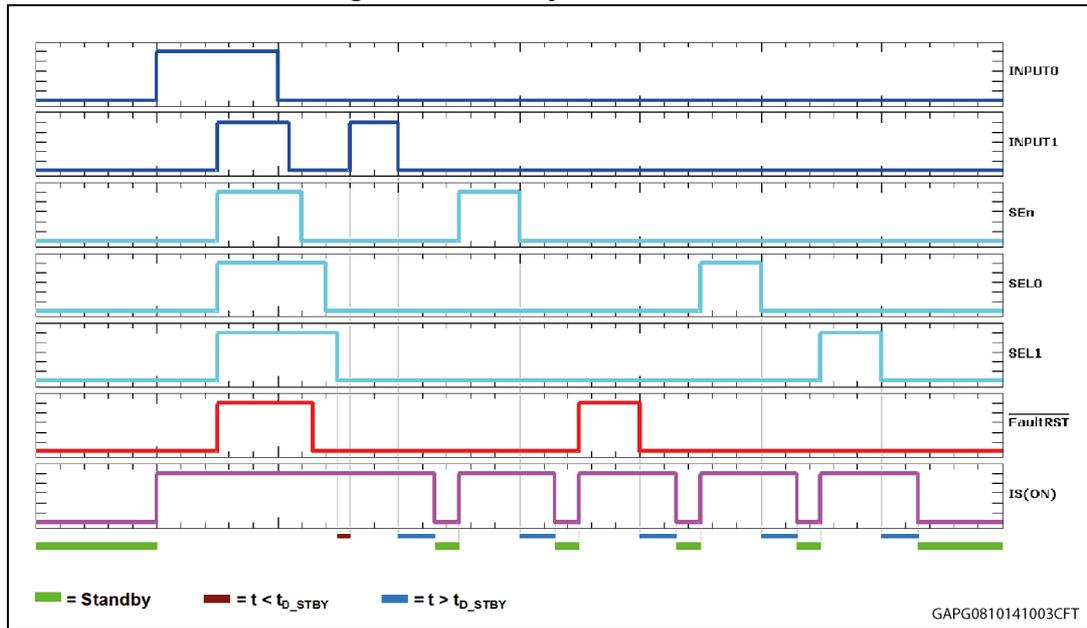
The device leaves the Standby mode when any of the above mentioned pins is set high (see Figure 30).
