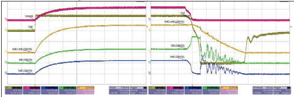
Figure 144. 2mH / 2.8Ω with external freewheeling (VND7040AJ, Ch.0 + Ch.1)
