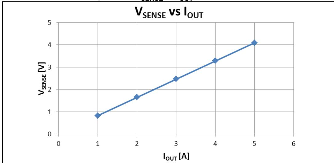
The trend is almost linear in the application range and then we can approximate the  $V_{SENSE}$  trend with the following equation:
