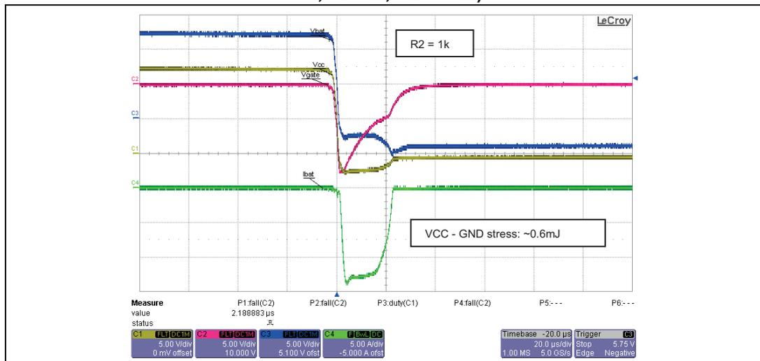
Figure 13 shows the example of an abrupt reverse battery test changing the polarity of the battery supply from 13.5 V to -4 V within a few us. The test setup used a 55 V/16 mΩ P-channel MOSFET with a gate resistor R2 = 1 kΩ. The total line impedance is measured with 82 mΩ in line with the requirements of LV 124:2009-10.
