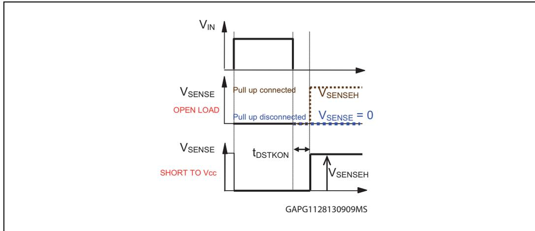
Figure 107. Open load/short to V<sub>CC</sub> detection in OFF state - delay after SE<sub>n</sub> is set from low to high
