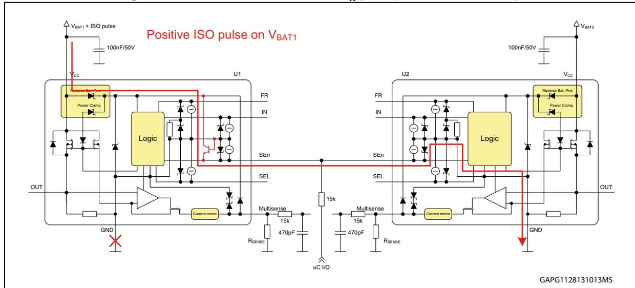
Direct connection of  $SE_n$  pins is not safe in the following cases:
