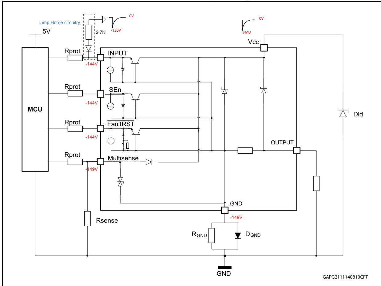
Besides, since the device input may be driven independently of the microcontroller by a separate HW, which is supplied directly from battery, it's mandatory to decouple the signal coming from the microcontroller to the one coming from the limp home circuitry, in order to avoid any backward supply of one circuit versus the other one. The decoupling is ensured by a signal diode, placed in series to the Limp Home path connected to the device input.
