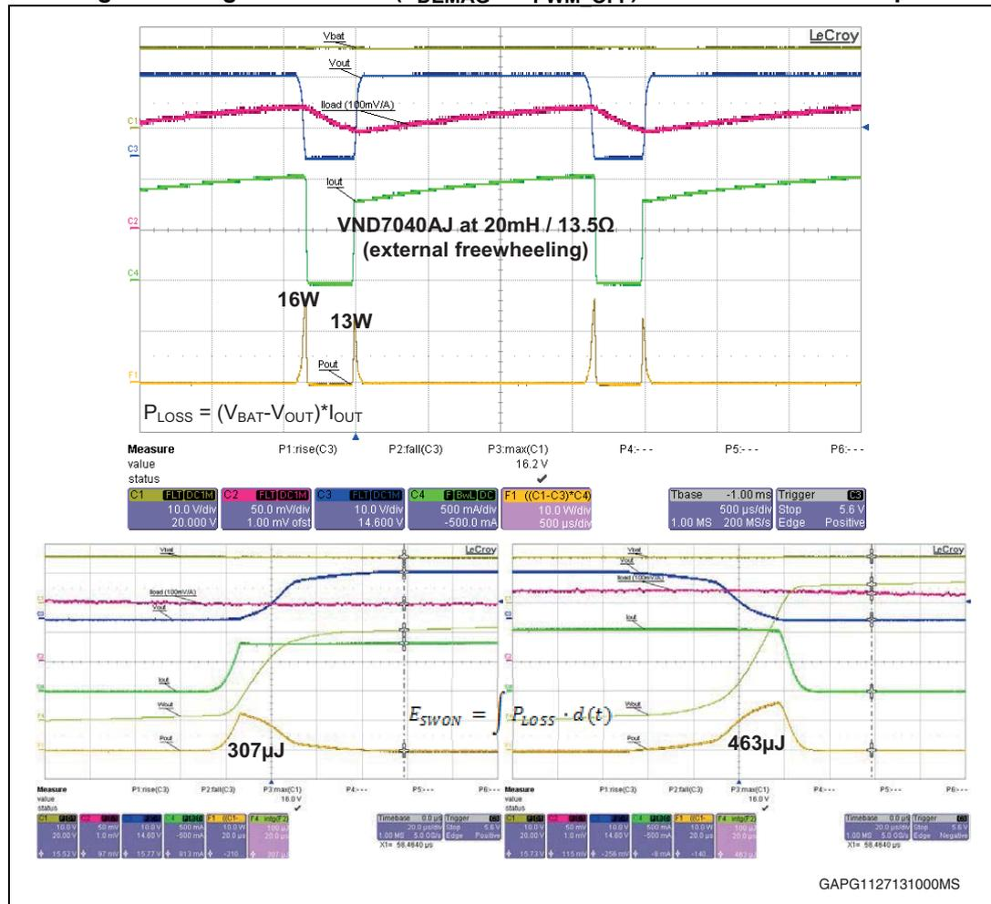
Measured losses (20 mH at 13.5 Ω):  $W_{ON} \sim 307 \mu J$  ( $I_{OUT} \sim 1 A$ )
