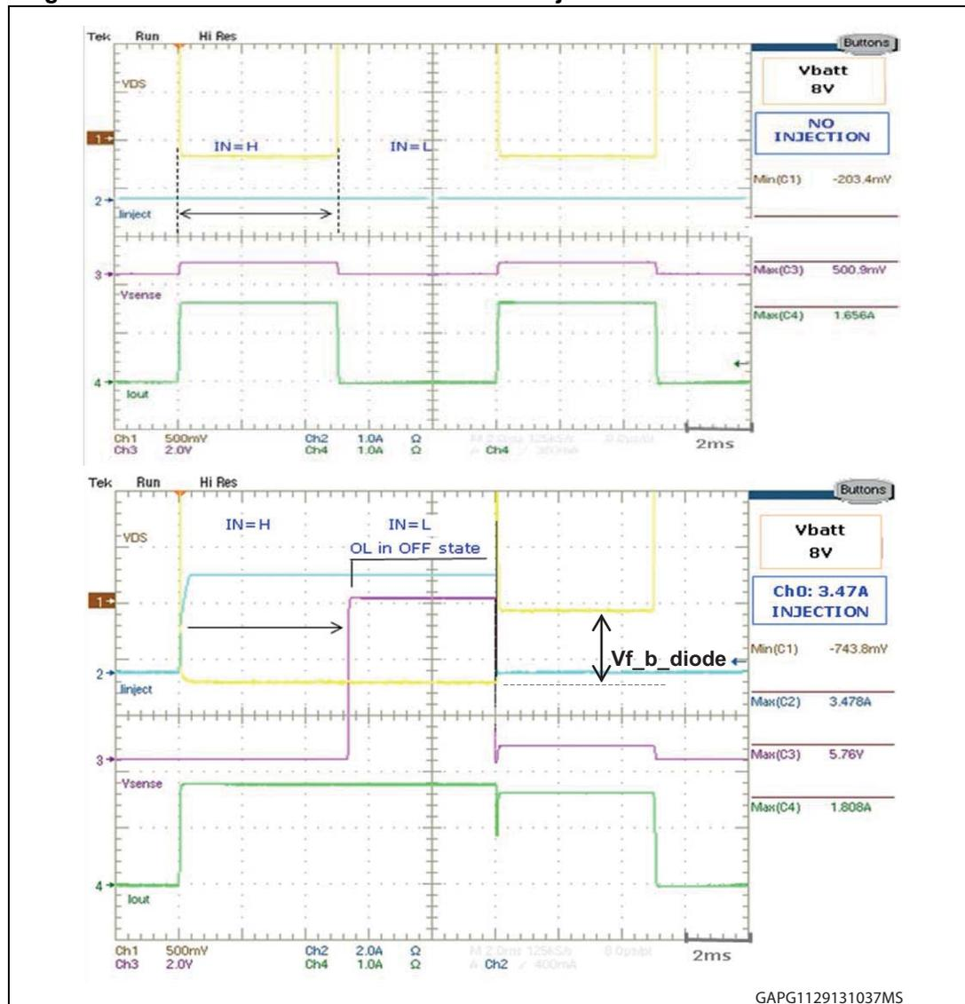
2. Device state: ChUT in PWM. Test execution: Increasing Inverse Current is injected in a channel (the ChUT) up to the  $I_{INVERSE}$  while the ChUT is driven ON
