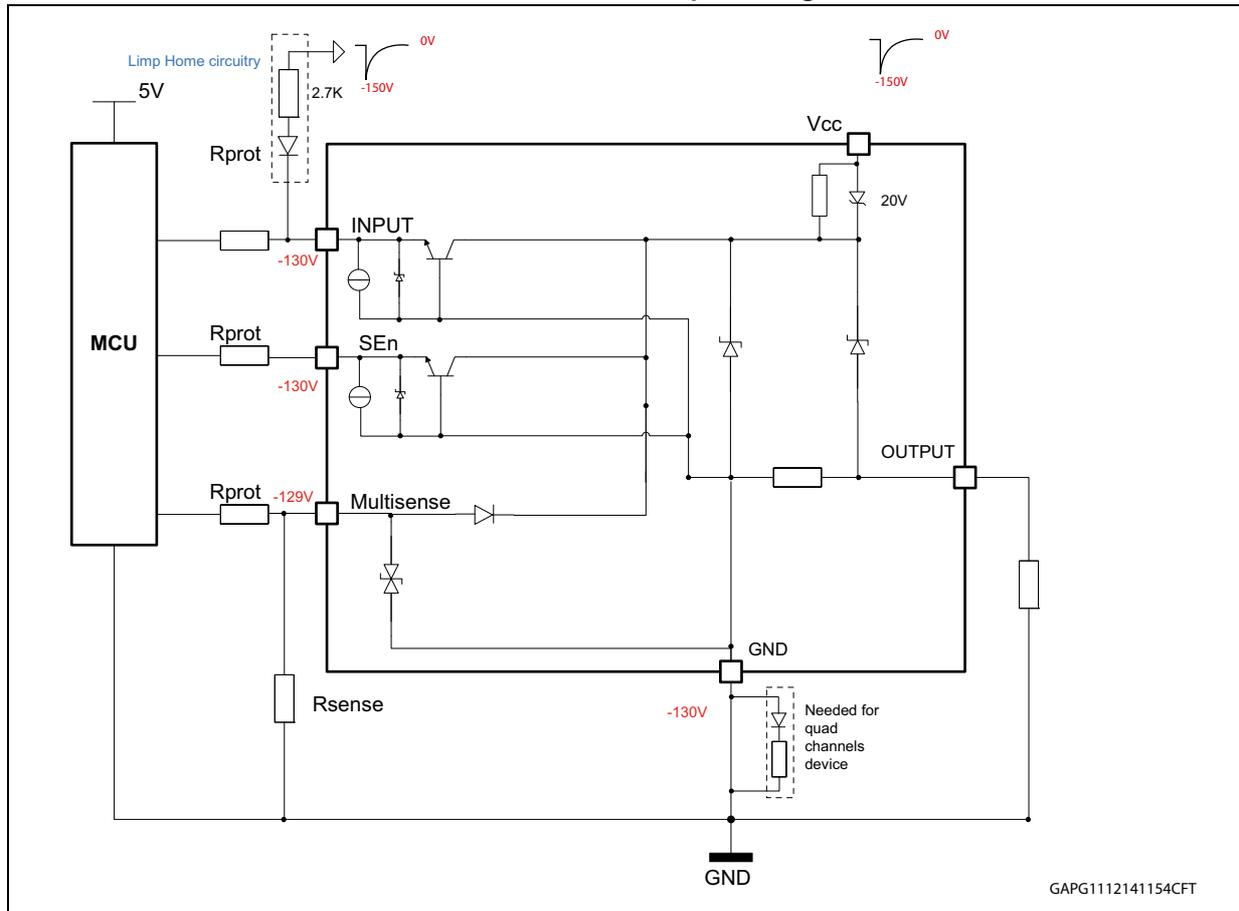
Besides, since the device inputs may be driven independently from the microcontroller by a separate HW (limp home feature), which is supplied directly from battery, it is mandatory to decouple the signal coming from the microcontroller to the one coming from the Limp home Circuitry, in order to avoid any backward supply of one circuit versus the other one. The decoupling is ensured by a signal diode, placed in series to the Limp Home path connected to the device input as shown in [Figure 22](#).
