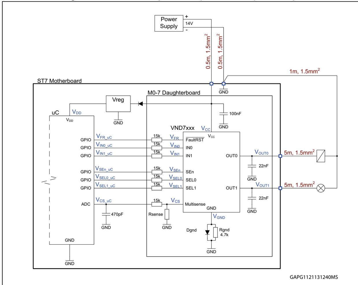
Figure 6. Measurement example ( $t_{\text{DEMAG}} > t_{\text{D\_STBY}}$ ) without GND resistor
