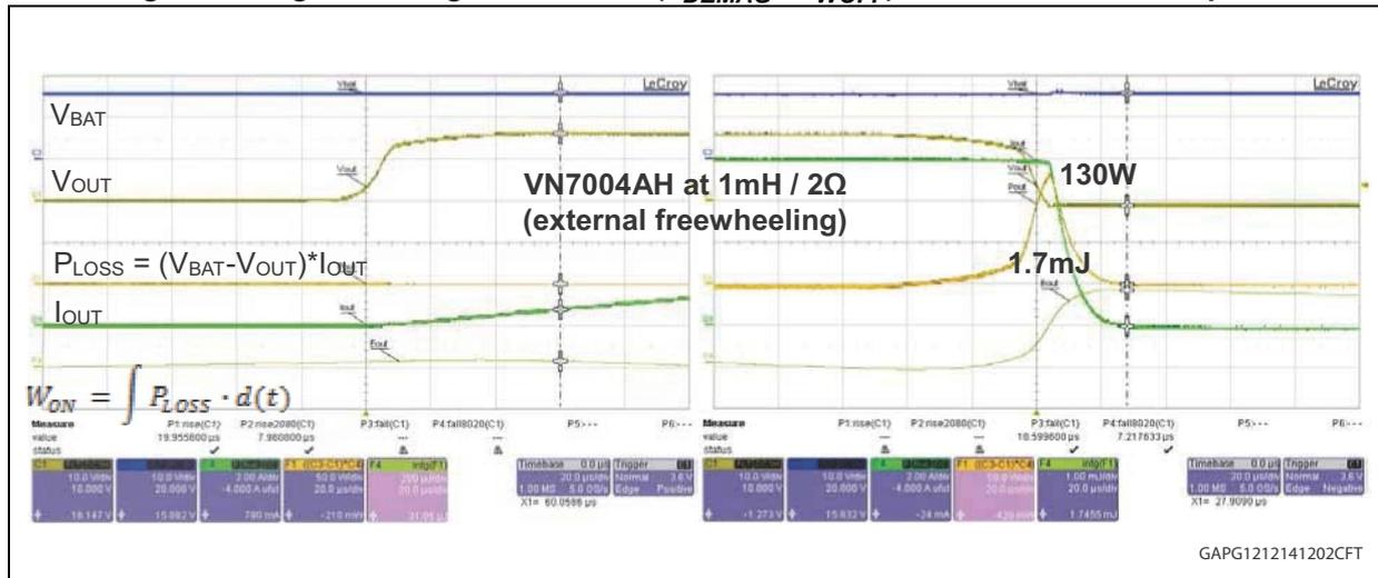
Measured losses (1 mH at 2  $\Omega$ ):  $W_{ON} \sim 0.04 \text{ mJ}$ ,  $W_{OFF} \sim 1.75 \text{ mJ}$
