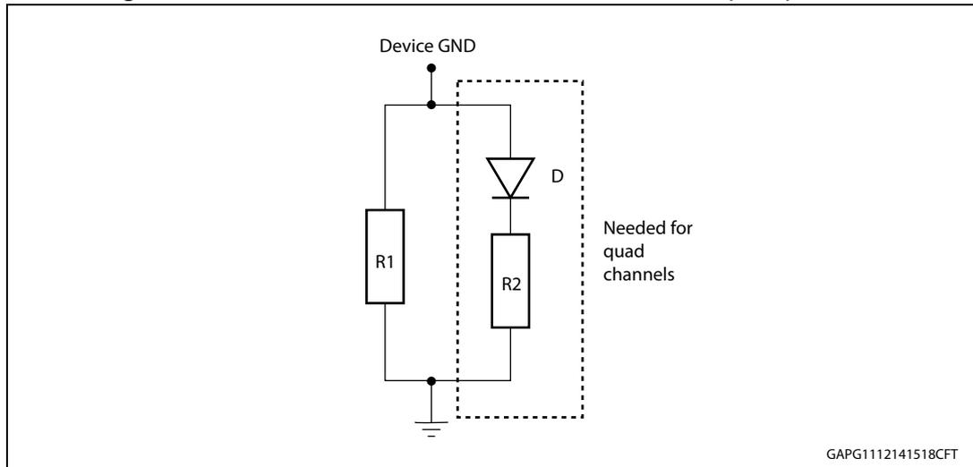
A second solution with an additional branch in parallel (R2 + low drop diode D) depends on specific considerations. The [Table 8](#) gives a suggestion according to the Hybrid device type and to the logic level of Input pin adopted.
