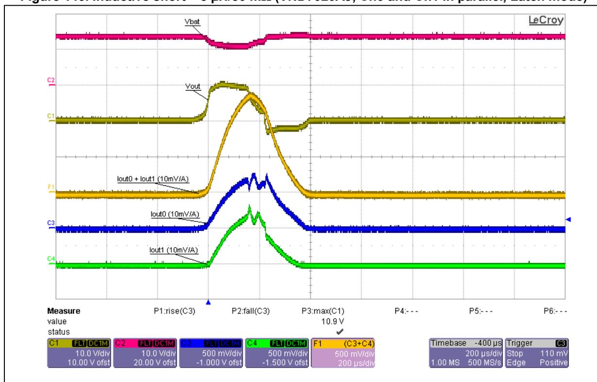
As seen from the measurement the device latches-off after the first power limitation pulse while the current among the channels is distributed almost equally.
