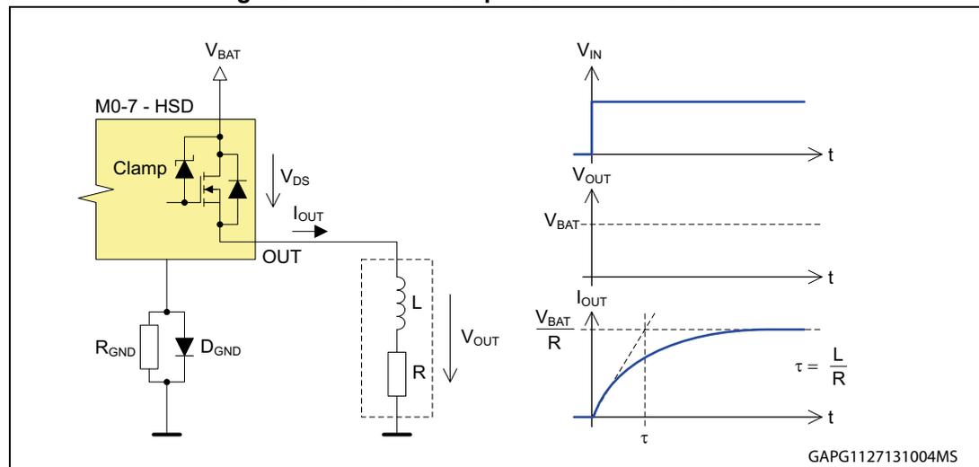
Figure 72. Turn-on example: VND7140AJ with inductive load (L = 260 mH, R = 81 Ω)
