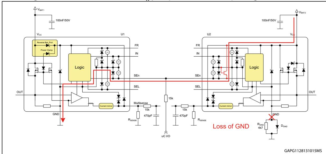
In configuration of separate supply lines where the GND connection of one device is lost, positive as well as negative ISO pulses on the associated supply line are not clamped anymore (considering no other devices connected to this supply line). If the transient voltage is big enough to activate involved structures, there could be unlimited current flow between both supply lines through SE<sub>n</sub> pins. This current could lead to malfunction or even failure of one or both of the HSDs.
