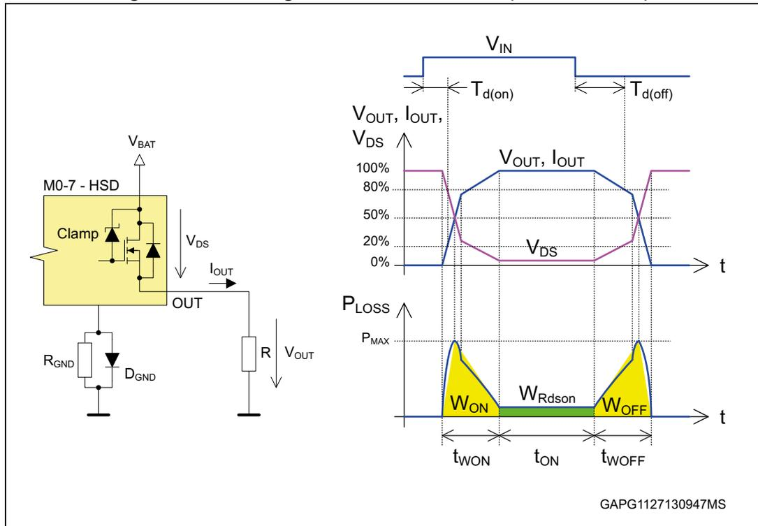
Considering resistive load, the maximum instantaneous power dissipation occurs at half of the nominal output voltage and half of the nominal load current. It is the point where the switch resistance matches the load resistance (maximum power transfer theorem, impedance matching).
