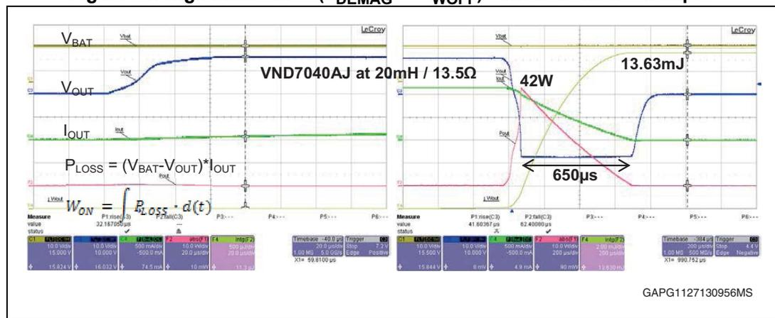
Measured T<sub>DEMAG</sub>: 6500 µs (633 µs calculated)
