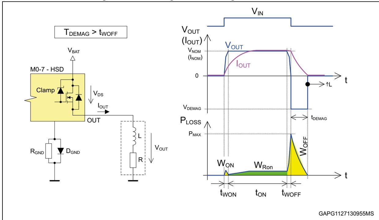
The above example explains a single turn-on / turn-off event. This means that zero load current is considered at the beginning of turn-on phase and nominal load current is considered at the beginning of turn-off phase.
