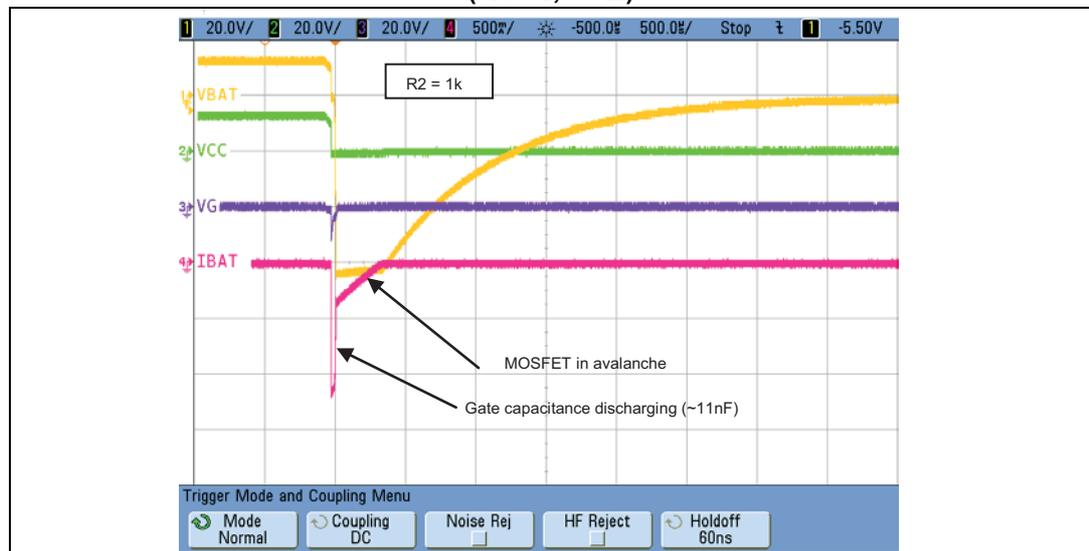
Figure 12 shows the example of a 55 V/16 m $\Omega$  P-channel MOSFET in the schematics as per Figure 11 submitted to ISO 7637-2:2004(E) pulse 1 transients. In order to limit the current in this experiment a 90  $\Omega$  generator resistor was chosen. As long as the P-channel
