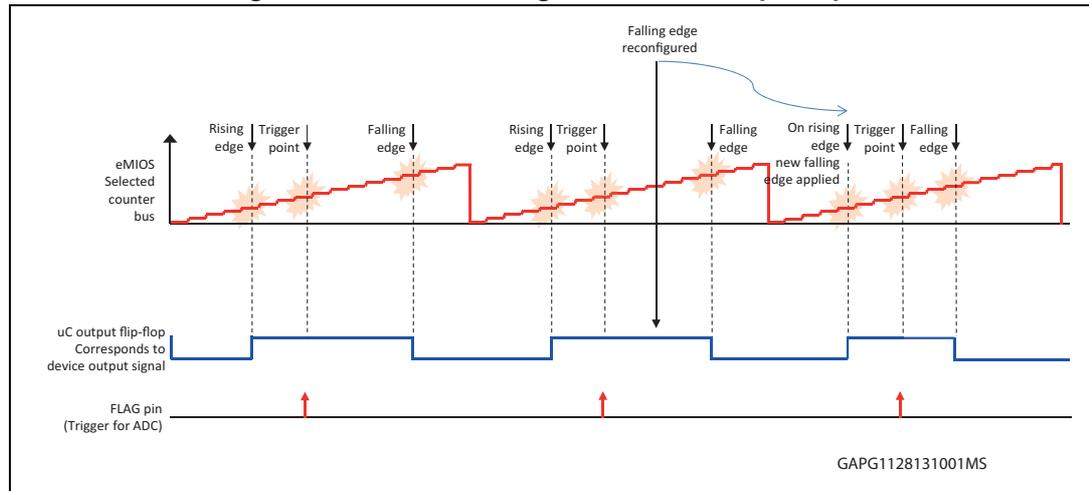
eMIOS block is able to control many channels applying independent configuration of rising, falling edge position (duty cycle), together with trigger, specifying sampling point for MultiSense signal. For example SPC560B64 - up to 2x31 channels are available for this purpose (other models can contain different number of eMIOS channels). These channels can be mapped directly to control INx signals of multiple HSDs.
