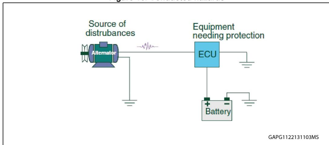
These hazards are generated by high current switching like relay contact, high current MOS or IGBT switches, ignition systems, etc. The electromagnetic field generated by these circuits directly affects lines or modules near the source of the electromagnetic radiation.
