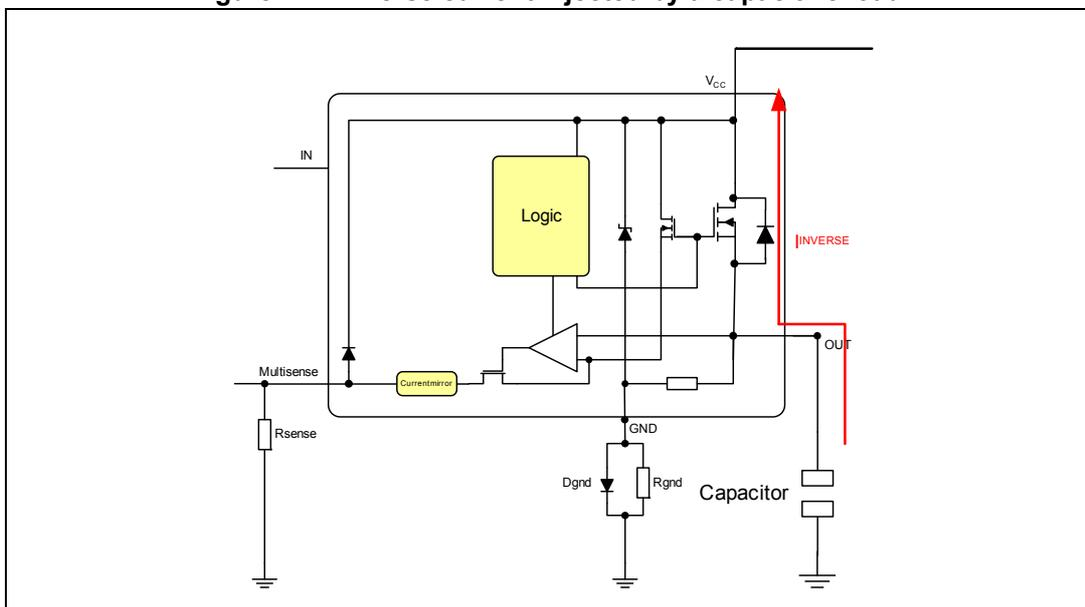
Figure 148. Inverse Current injected by an inductive load in the high-side driver of an H-Bridge
