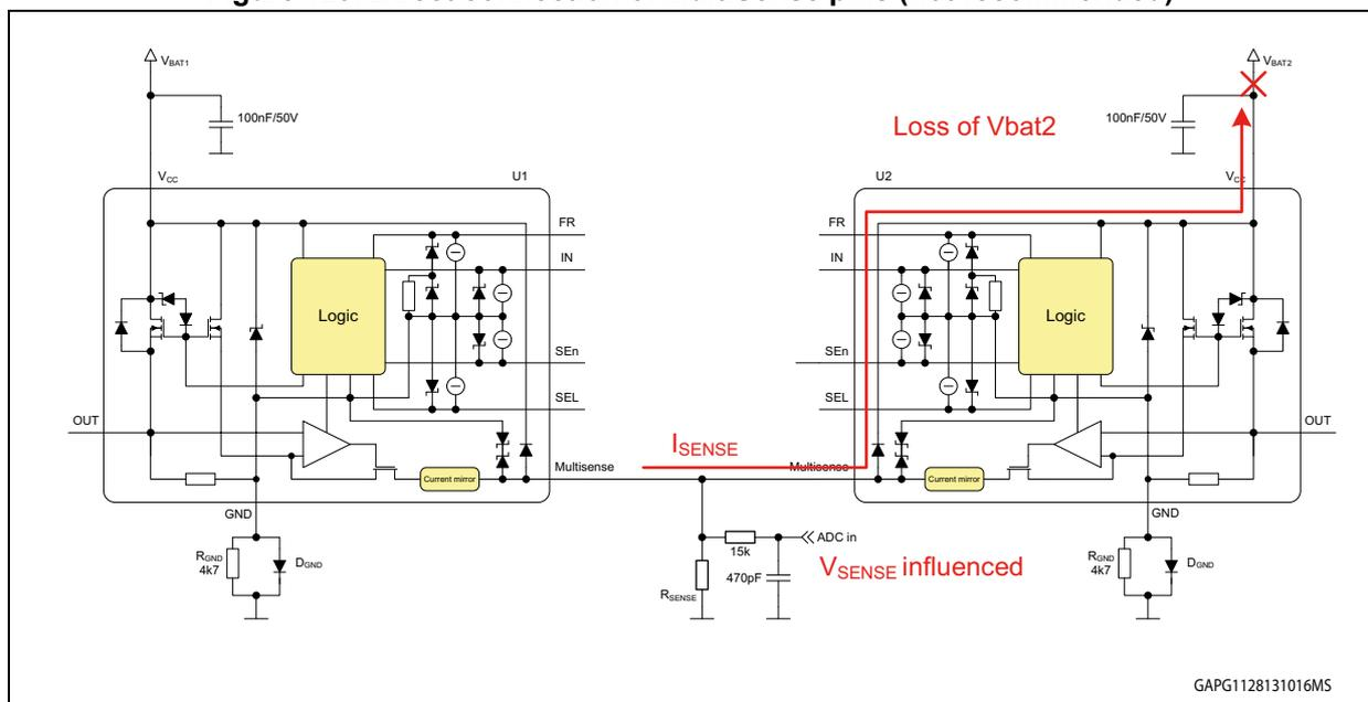
Direct connection of MultiSense pins is not safe in the following cases:
