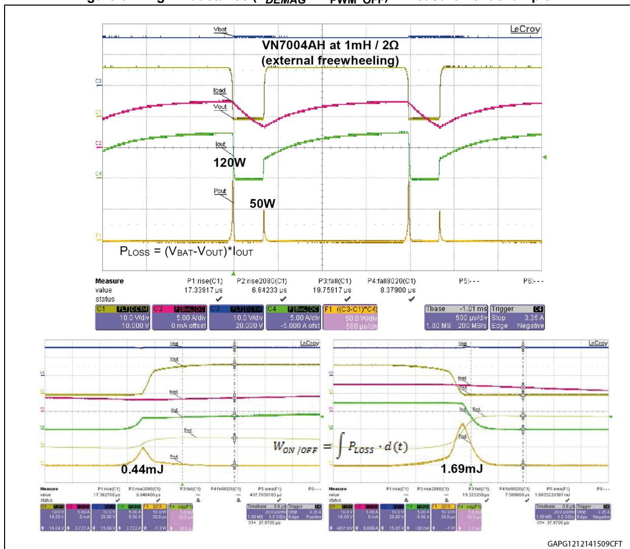
Measured losses (1 mH at 2 Ω):  $W_{ON} \sim 0.44$  mJ,  $W_{OFF} \sim 1.69$  mJ
