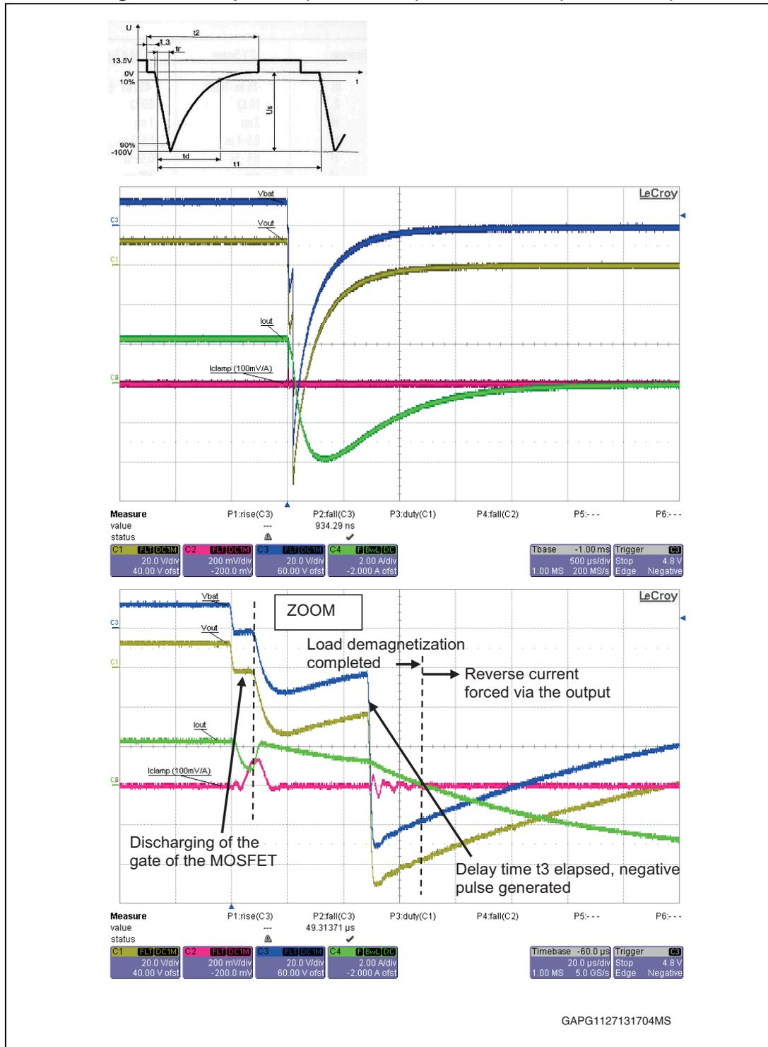
Figure 82. Loss of V<sub>CC</sub>, 2 mH / 5.5 Ω (VND7040AJ)
