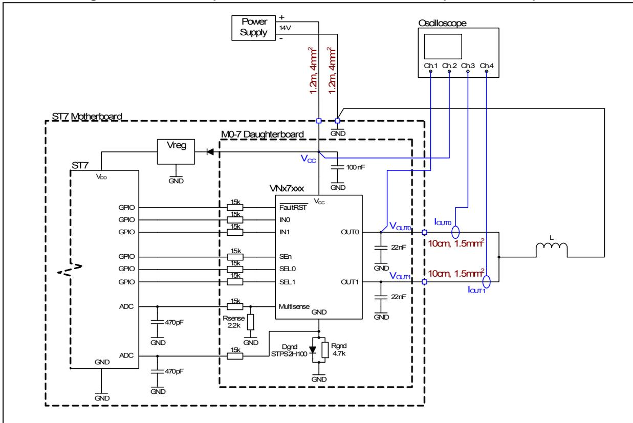
Figure 146. Inductive short – 5  $\mu$ H/50 m $\Omega$  (VND7020AJ, Ch0 and Ch1 in parallel, Latch mode)
