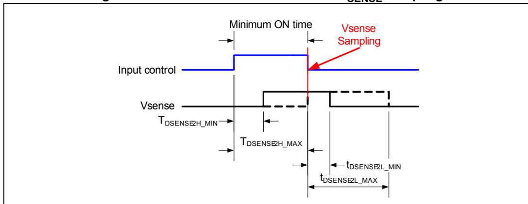
$t_{DSENSE2H} \sim 250 \mu s$  (maximum datasheet value)
