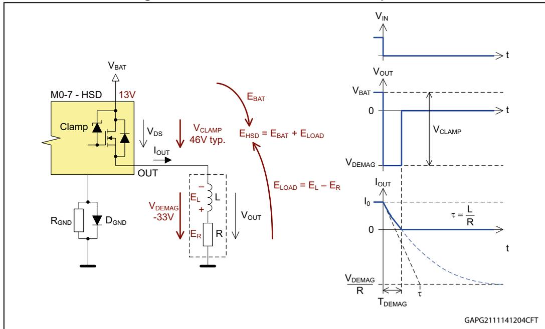
The load current decays exponentially (linearly if  $R \rightarrow 0$ ) and reaches zero when all energy stored in the inductor is dissipated in the HSD and the load resistance.
