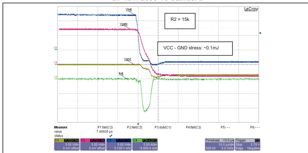
Figure 10 shows an example of an abrupt reverse battery test changing the polarity of the battery supply from 13.5 V to -4 V within a few  $\mu$ s. The test setup used a 100 V/100 mΩ N-channel MOSFET with a gate resistor  $R2 = 15$  kΩ. The total line impedance is measured with 82 mΩ in line with the requirements of LV 124: 2009-10.
