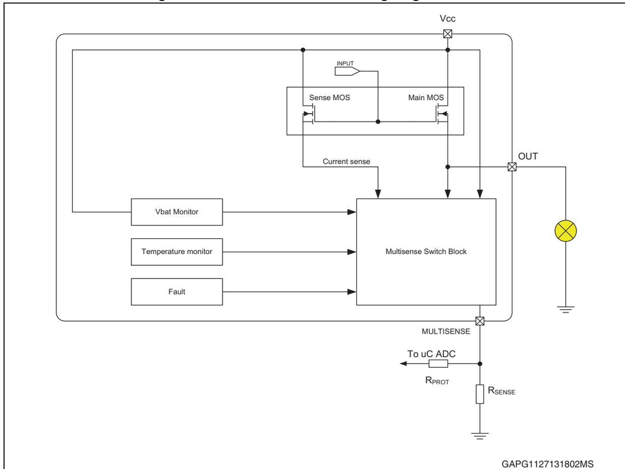
In General, the MultiSense output signal operates for  $V_{CC} < 24\text{ V}$
