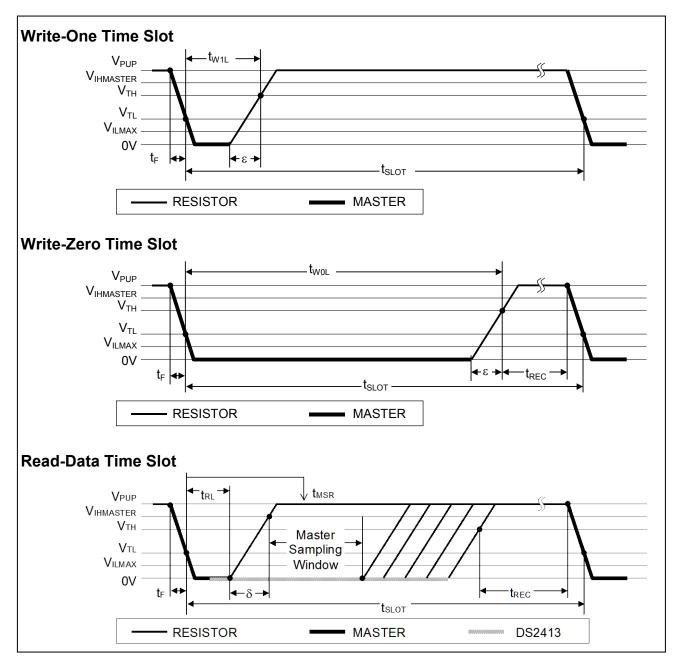
Figure 12. Read/Write Timing Diagram
