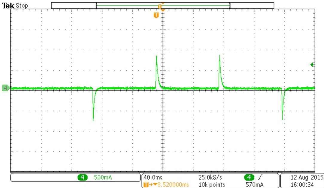
Figure 35. Motor Phase Current With 12-Hz IPD Clock
