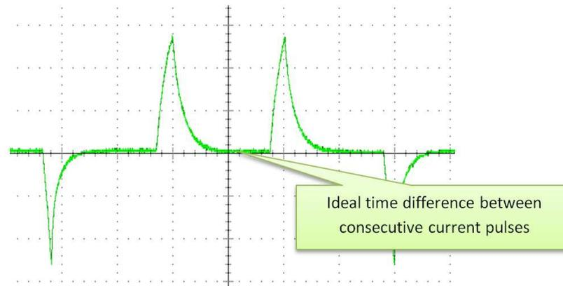
Figure 21. Current Waveform During IPD Process With Optimized 'IPD Clock' Frequency
