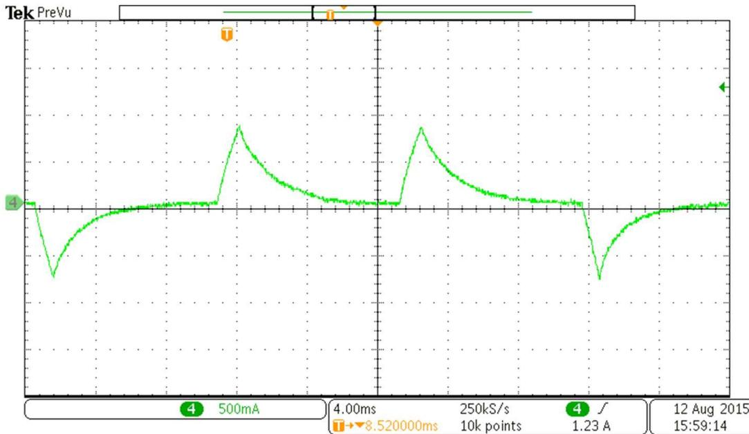
**Figure 41. Motor Phase Current With 95-Hz IPD Clock**
