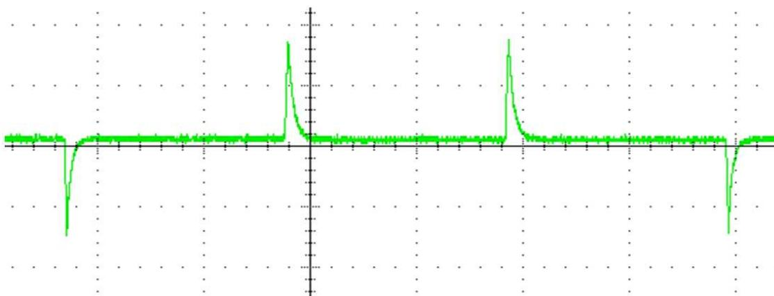
Figure 32. Motor Phase Current During Brake Mode
