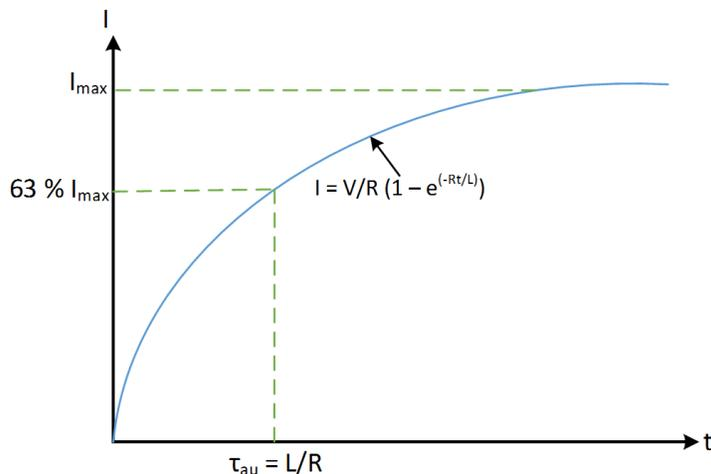
**Figure 24. Step Response of Series LR Circuit**
