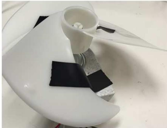
**Figure 25. Align and Lock Shaft of Motor**
