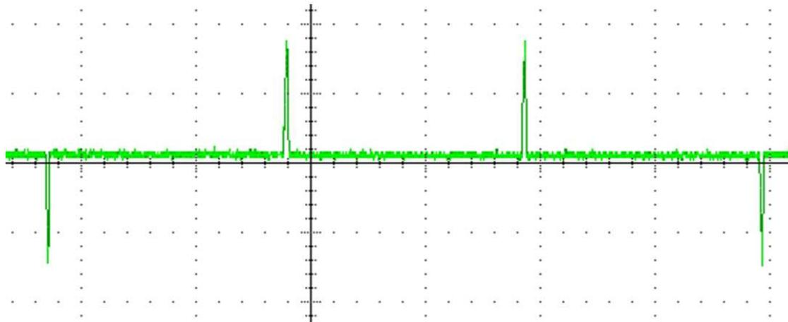
**Figure 33. Motor Phase Current During Tristate Mode**
