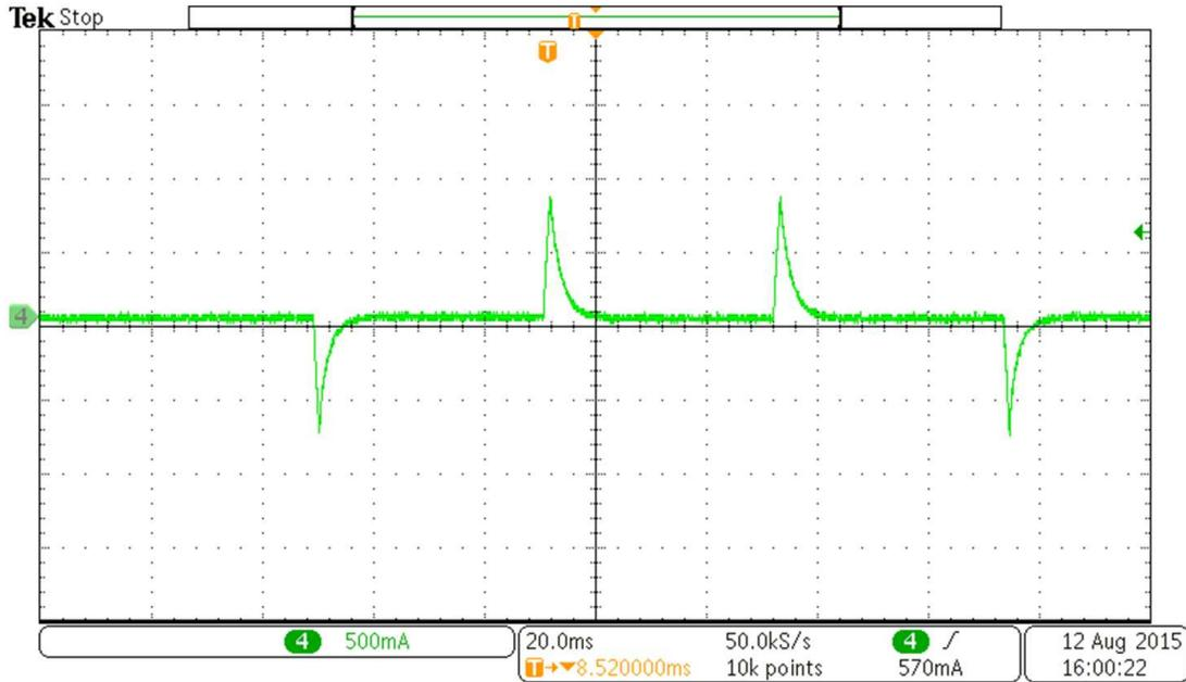
Figure 37. Motor Phase Current With 24-Hz IPD Clock
