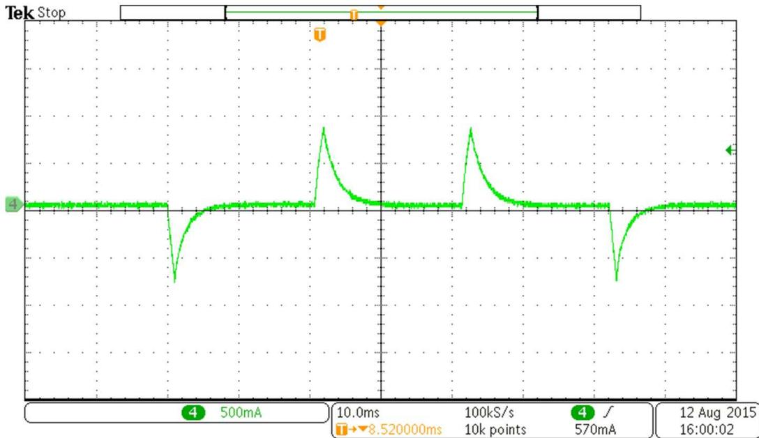
Figure 39. Motor Phase Current With 47-Hz IPD Clock
