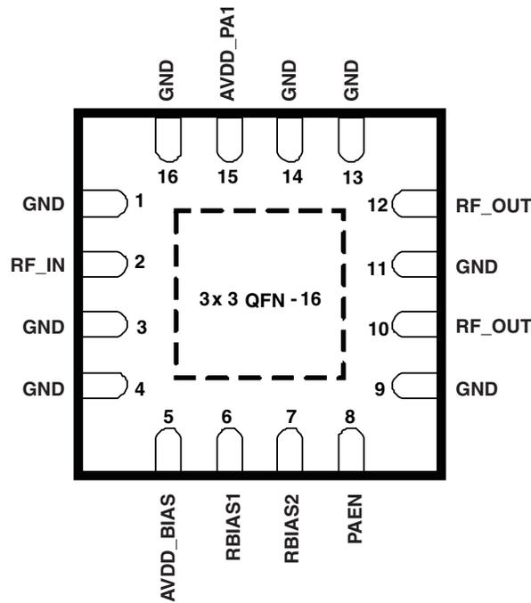
**Figure 1. CC2595 Pinout**
