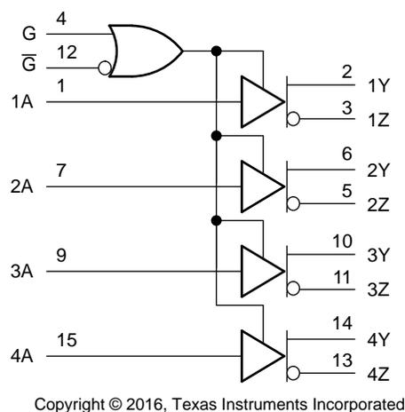
**Figure 7. Logic Diagram**
