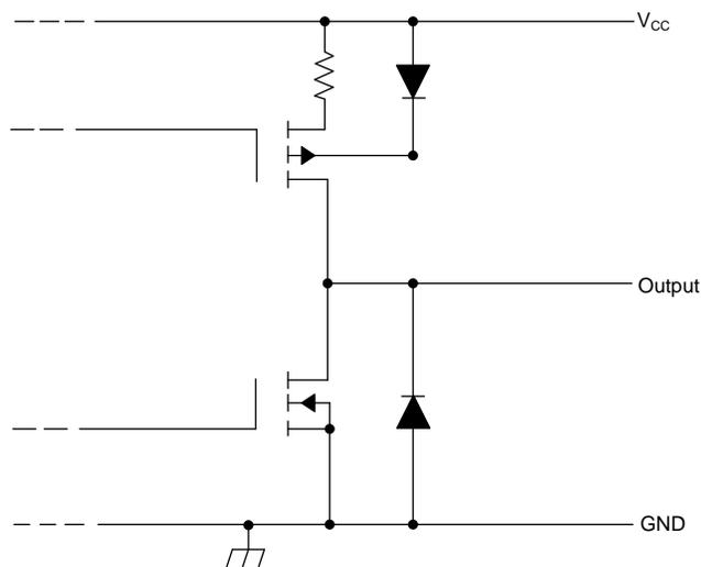
Figure 9. Typical of Each Driver Output Schematic
