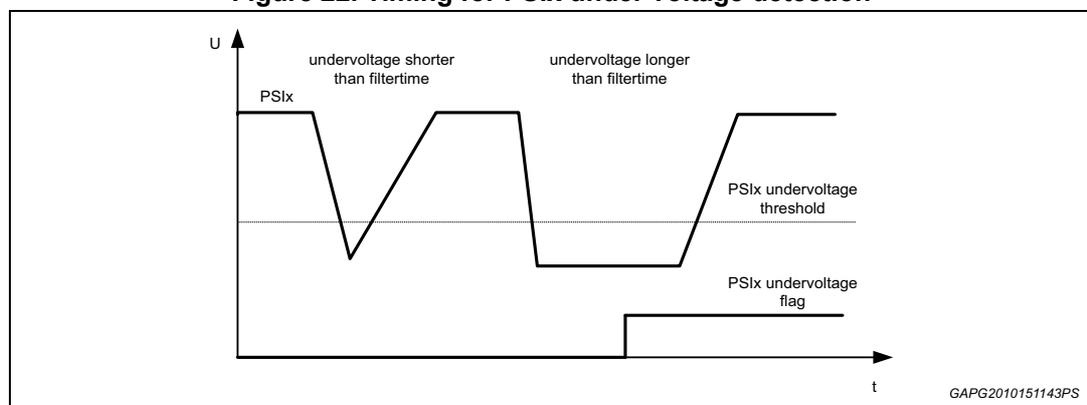
The PSIx lines (sensor supply lines) are monitored for under voltage if the PSIx line is switched on.
