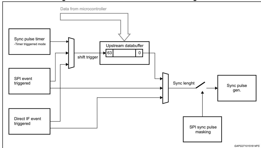
The synchronization bits in the ECU to sensor communication must be programmed in the upstream data buffer by the microcontroller.
