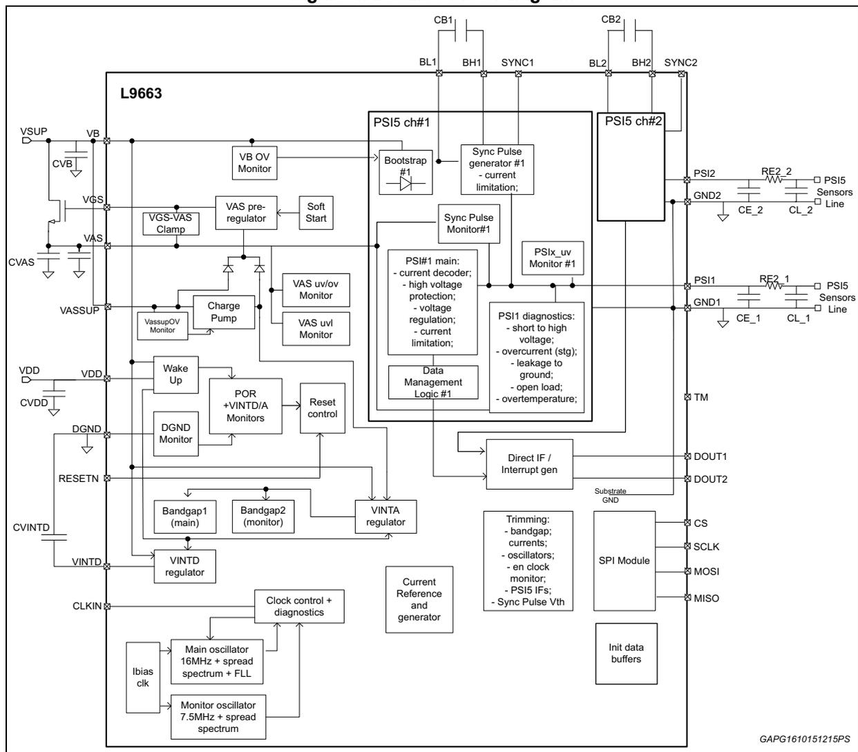
The high supply voltage of the IC can be a battery or a regulated voltage provided by the ECU.
