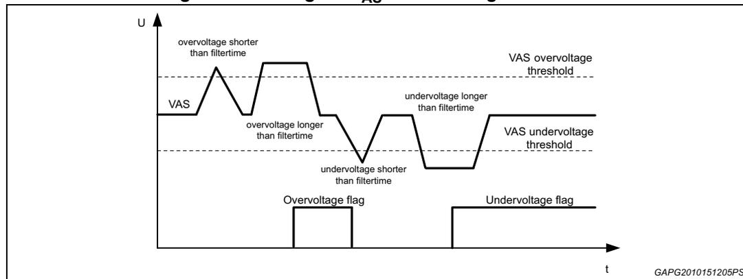
If the  $V_{AS}$  voltage is lower than the under voltage threshold for longer than the filter time, the SPI bit  $VAS\_UV$  in SR1 reg is set to '1' and it is latched and cleared upon read.
