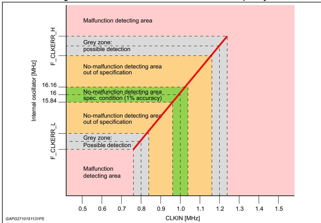
If the CLKIN is stuck the device behavior is shown in the figure below: in this case during the detection time the tolerance is still inside the 1% tolerance until the device enters reset (T\_CKERD max 260 μs).
