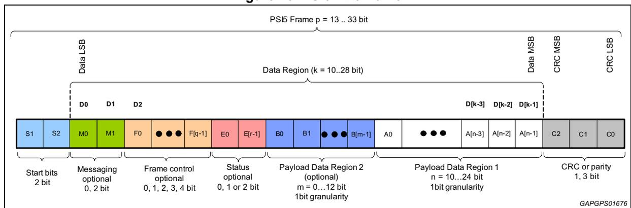
In case of PSI5 v2.x, the length of the data region can vary between  $k = 10 \dots 28$  bits, with 1-bit granularity. The data region can be split into the following fields and regions:
