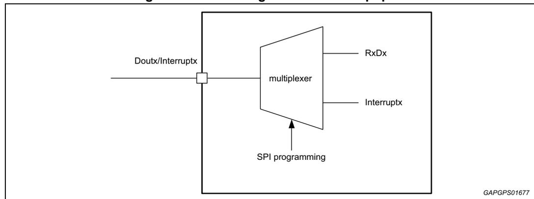
After reset, the output pin is configured as DOUTx.
