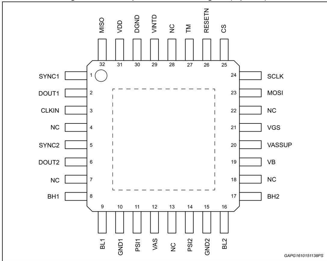
**Note:** The exposed pad is electrically shorted to the substrate and to pins GND1 and GND2. These three nodes have to be kept shorted on the application.
