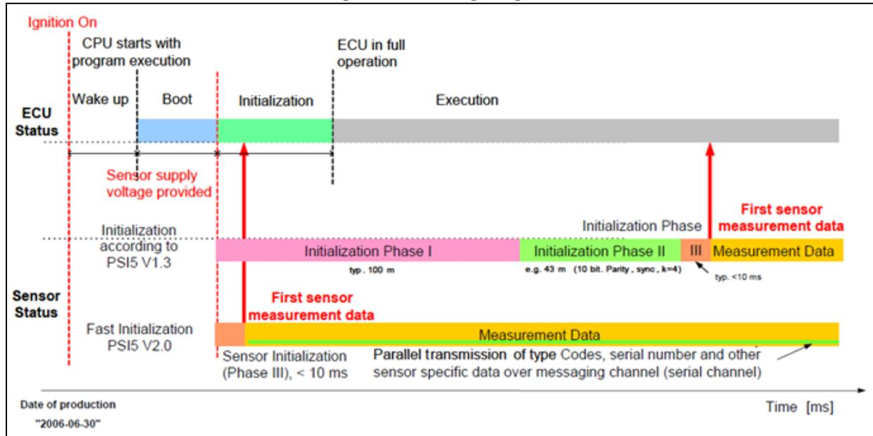
After the activation of an interface, the transceiver IC can check for incoming sensor initialization data on that interface and store the data for further processing. This behavior is triggered by the configuration bit READ\_INIT\_DATA on that channel.
