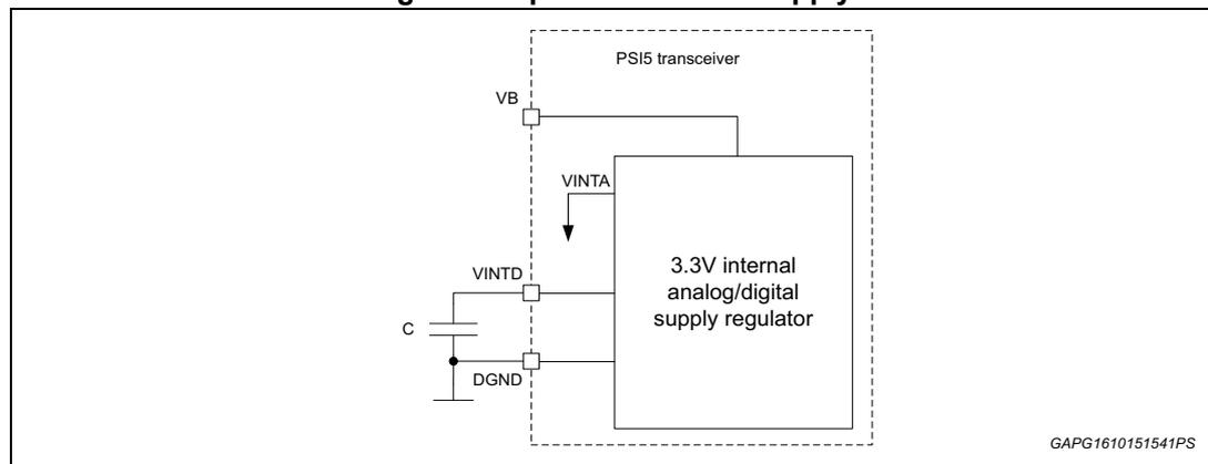
A ceramic capacitor with a typical capacitance of 100 nF is required as a blocking capacitor close to the pins  $V_{DD}$  and  $V_B$ .
