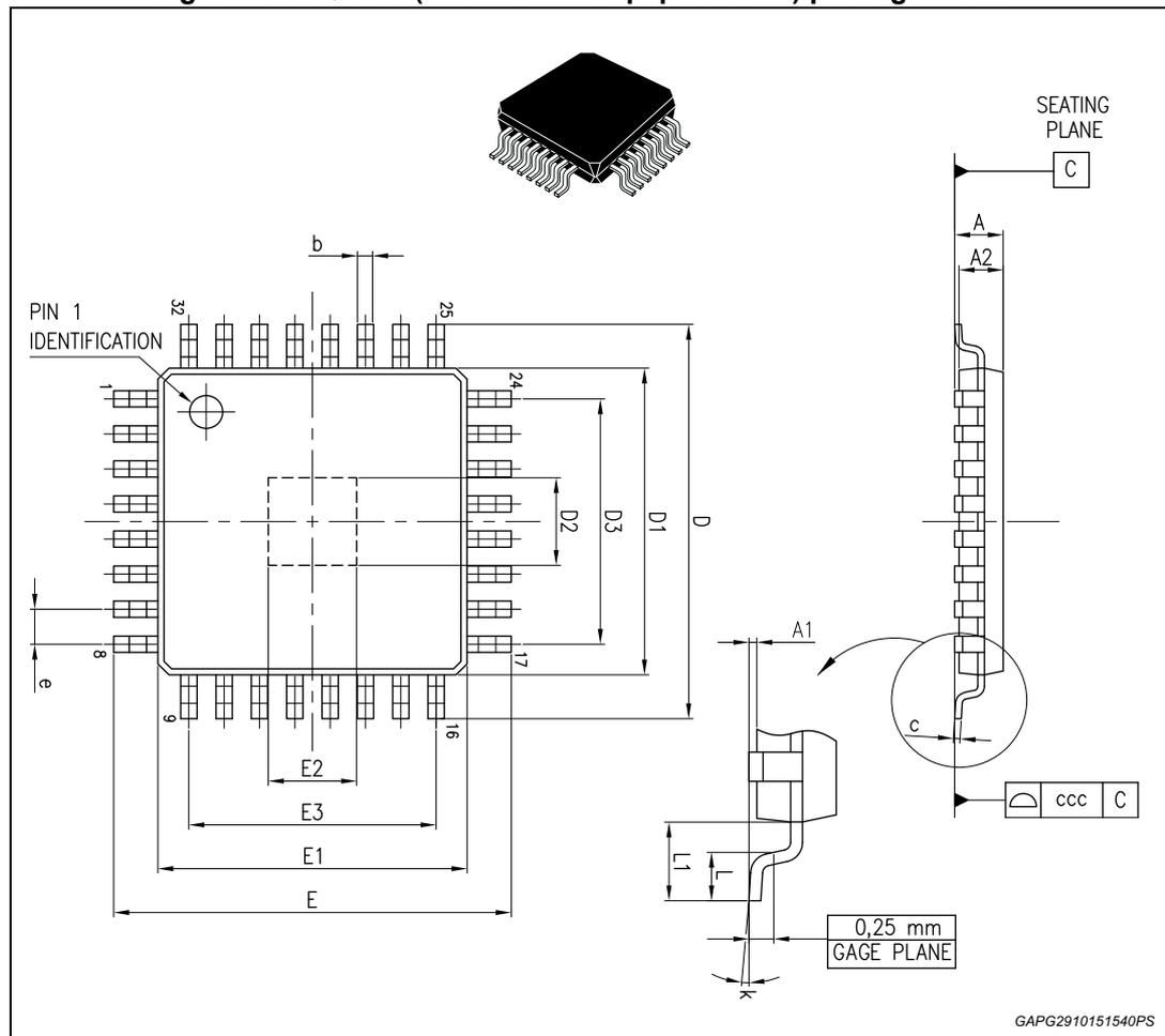
Table 28. TQFP32 (7x7x1.0 mm exp. pad down) package mechanical data
