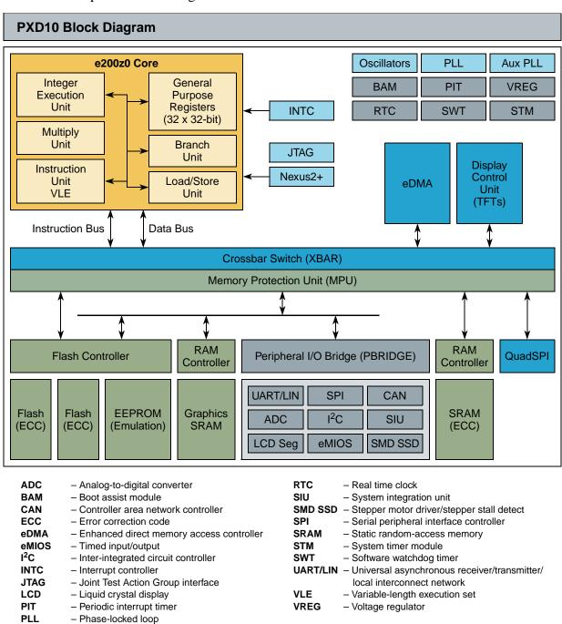
Figure 1. PXD10 Block Diagram
