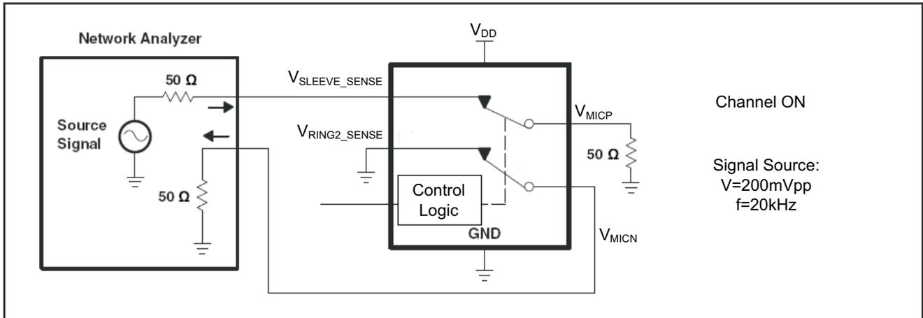
Figure 9. Channel Separation
