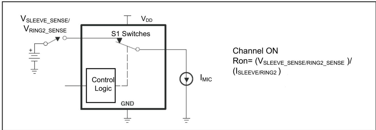
Figure 4. S1 Switch On Resistance Measurement
