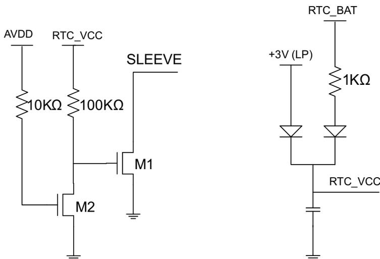
With the use of this circuitry, the SLEEVE pin will be pulled down to GND by the RTC\_VCC power source. The RTC\_VCC power source is generated by the Real Time Clock source running off a small on-board battery (RTC\_BAT) that is kept running even in G3 mode. With SLEEVE pin pulled down to GND, ground return path is established for the speaker and noises will be eliminated. Diodes are added from RTC\_BAT to +3V (LP) to prevent leakage when system is turning on.
