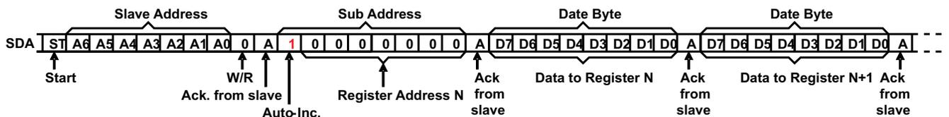
Figure 14. Burst Data Write to Multiple Registers
