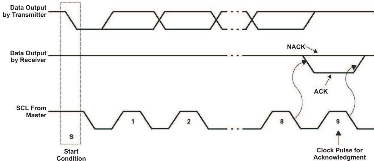
Figure 12. Acknowledgment on I<sup>2</sup>C Bus
