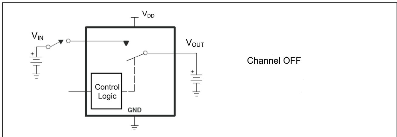
Figure 5. Switch Off Leakage Current Measurement
