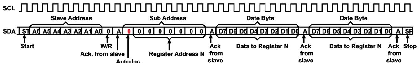
Figure 13. Repeated Data Write to a Single Register
