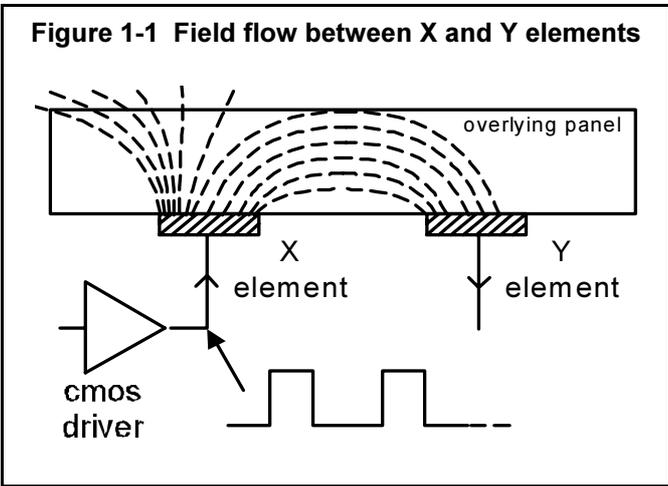
The 60320 uses burst-mode charge transfer methods pioneered and patented by Quantum, including charge cancellation methods which allow for a wide range of key sizes and shapes to be mixed together in a single keypad. These features permit the construction of entirely new classes of keypanels never before contemplated, such as touch-sliders, back-illuminated keys, and arbitrary shape keypanels, all at very low cost.
