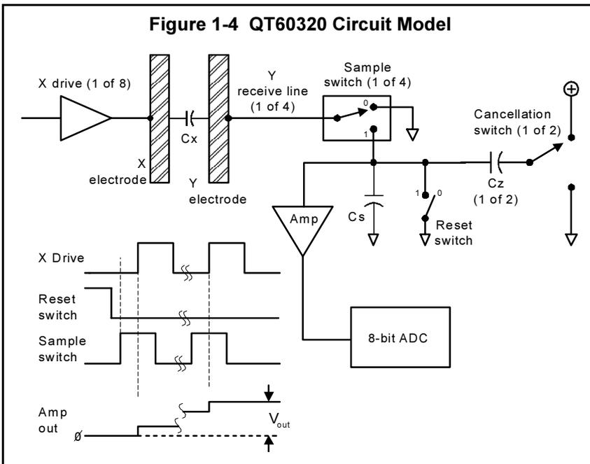
groupings of bursts; a 4-pole analog switch acts as the sample switch for all 4 Y lines. At the intersection of each X and Y line is an interdigitated electrode set as shown in Figure 1-6. Typically the outermost electrode is connected to X and the inner electrode connected to Y. Remaining Y lines not being sampled are grounded.
