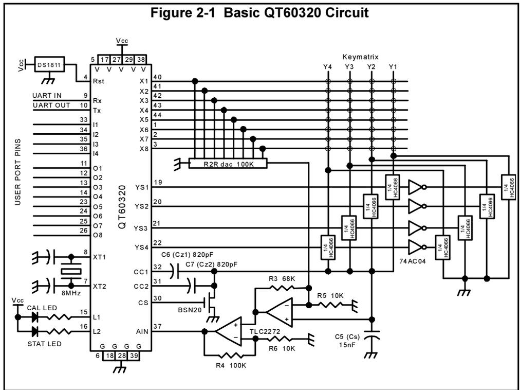
If there is a large amount of coupling between X and Y lines, and where burst length 'n' is set to a high number, charge accumulation on Cs may reach a point where the ladder DAC can no longer offset the signal back into the ADC's usable range. In this case the circuit will employ one or two of the Cz capacitors to 'knock back' or cancel the charge accumulated on Cs; each Cz will cancel charge in a discrete step as required.
