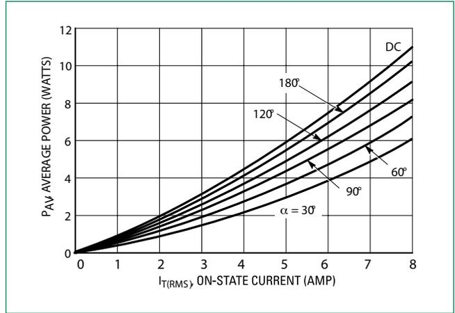
**Figure 3. On-State Characteristics**
