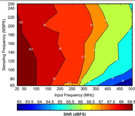
**Figure 46. SNR Contour (0-dB Gain, Applies to ADS41B29)**
