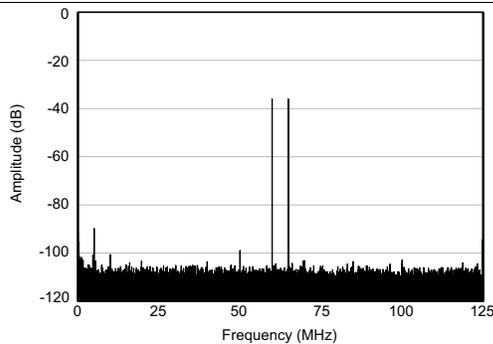
Figure 5. FFT for Two-Tone Input Signal
