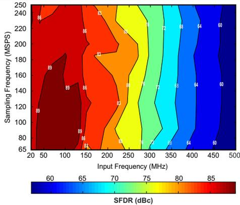
**Figure 42. SFDR Contour (0-dB Gain, Applies to ADS41Bx9)**
