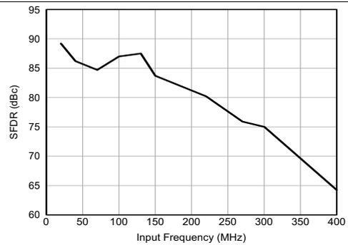
Figure 6. SFDR vs Input Frequency
