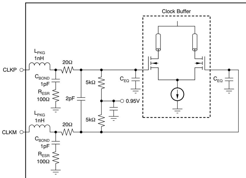
NOTE:  $C_{EQ}$  is 1 pF to 3 pF and is the equivalent input capacitance of the clock buffer.
