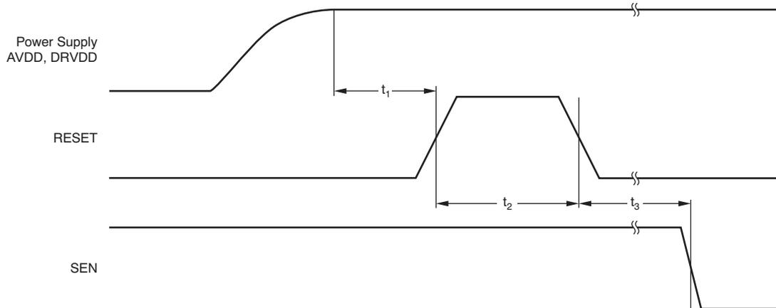
NOTE: A high pulse on the RESET pin is required in the serial interface mode in case of initialization through hardware reset. For parallel interface operation, RESET must be permanently tied high.
