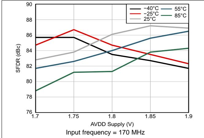
Figure 31. SFDR Across Ambient Temperature vs AVDD Supply
