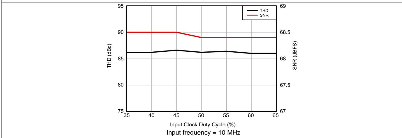
Figure 35. Performance Across Input Clock Duty Cycle
