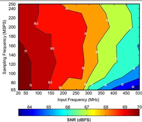
**Figure 44. SNR Contour (0-dB Gain, Applies to ADS41B49)**
