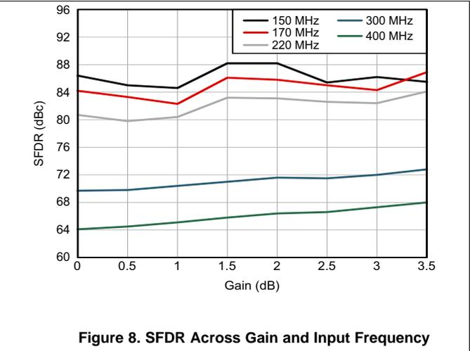
**Figure 8. SFDR Across Gain and Input Frequency**
