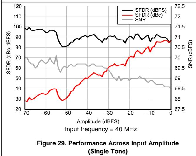
**Figure 29. Performance Across Input Amplitude (Single Tone)**
