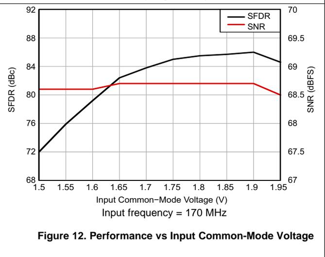
**Figure 12. Performance vs Input Common-Mode Voltage**
