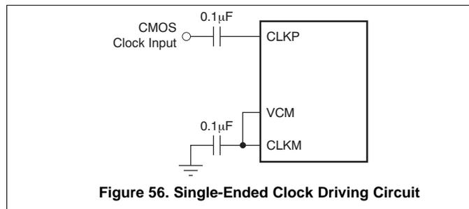
Figure 56. Single-Ended Clock Driving Circuit
