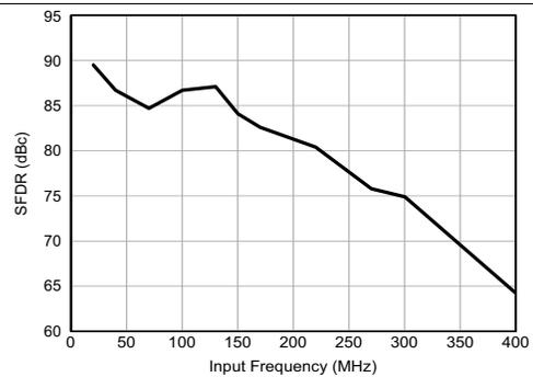
**Figure 24. SFDR vs Input Frequency**
