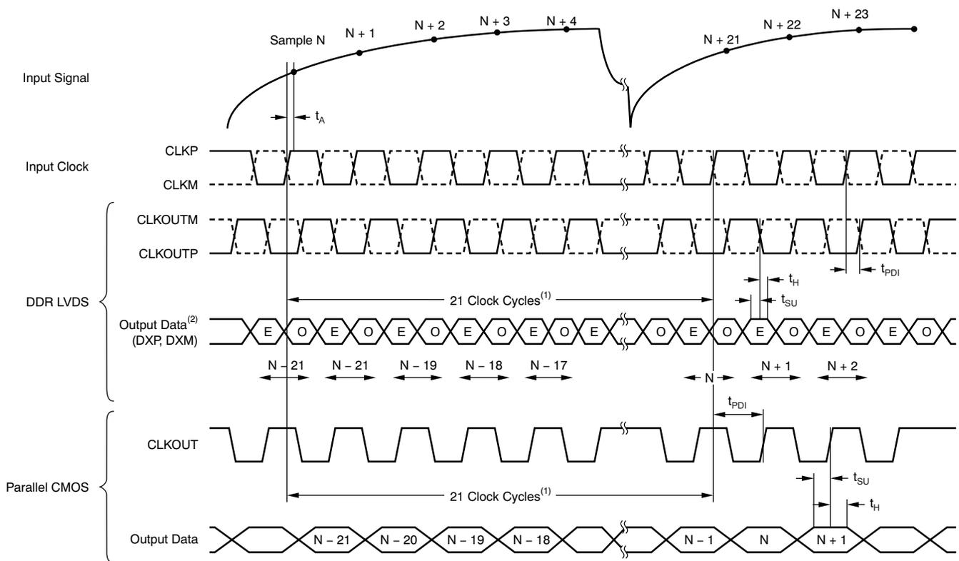
(1) At higher sampling frequencies,  $t_{PDI}$  is greater than one clock cycle which then makes the overall latency = ADC latency + 1.
