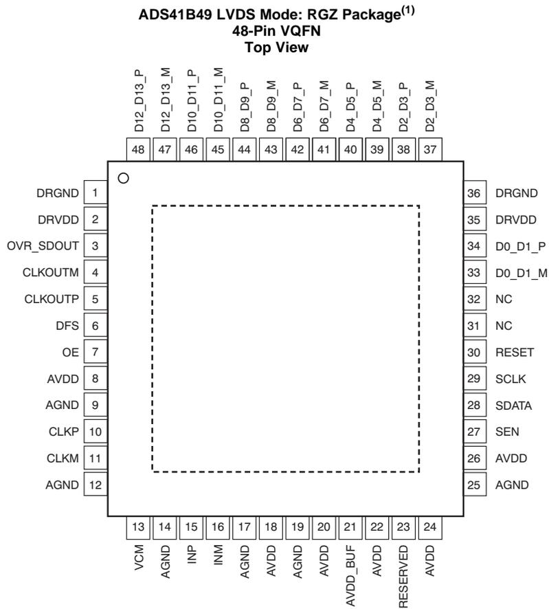
(1) The PowerPAD™ is connected to DRGND.
