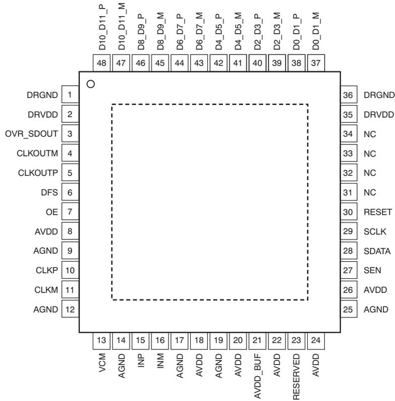
(1) The PowerPAD is connected to DRGND.
