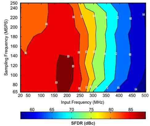
**Figure 43. SFDR Contour (3.5-dB Gain, Applies to ADS41Bx9)**
