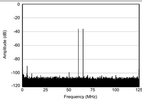
**Figure 23. FFT for Two-Tone Input Signal**
