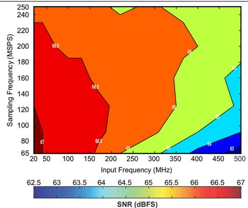
**Figure 45. SNR Contour (3.5-dB Gain, Applies to ADS41B49)**
