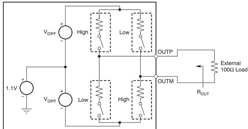
NOTE: Use the default buffer strength to match 100-Ω external termination ( $R_{OUT} = 100 \Omega$ ). To match with a 50-Ω external termination, set the LVDS STRENGTH bit ( $R_{OUT} = 50 \Omega$ ).
