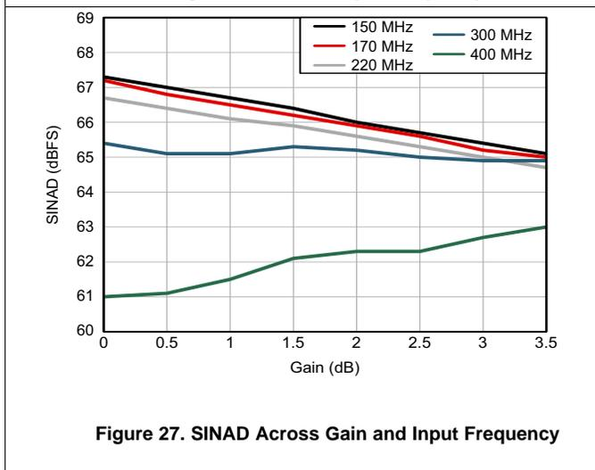
**Figure 27. SINAD Across Gain and Input Frequency**
