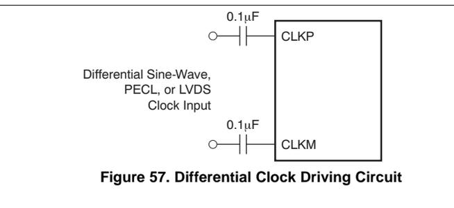
Figure 57. Differential Clock Driving Circuit
