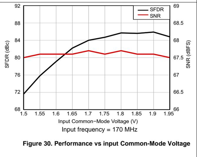
**Figure 30. Performance vs input Common-Mode Voltage**
