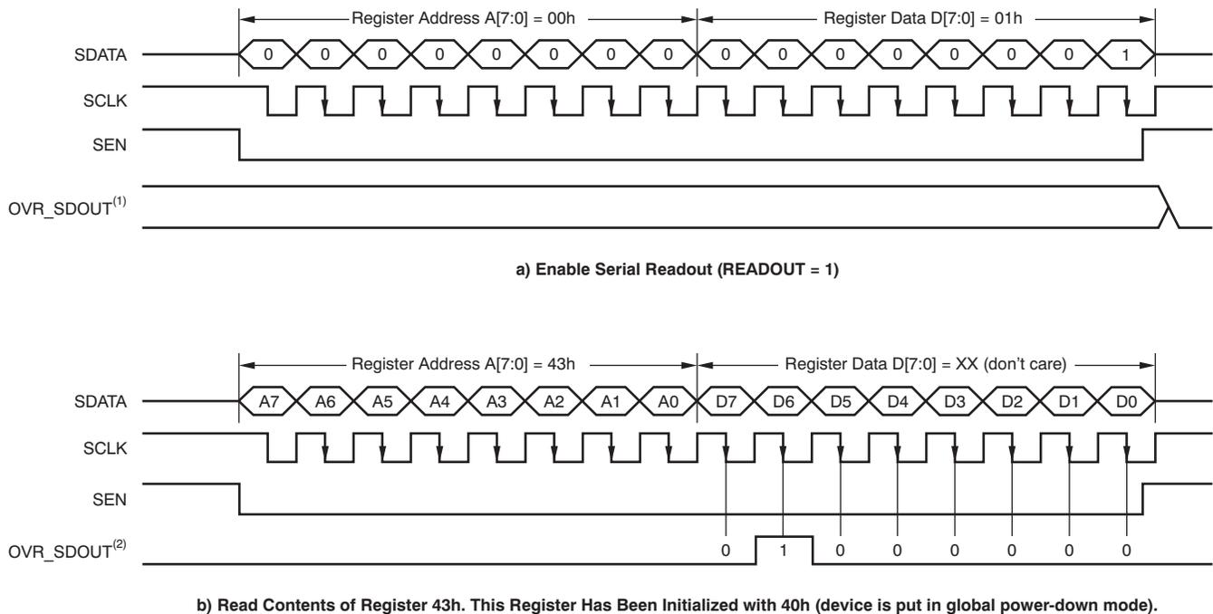
(1) The OVR\_SDOUT pin functions as OVR (READOUT = 0).
