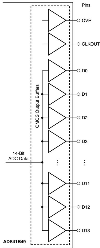
Figure 63. CMOS Output Interface
