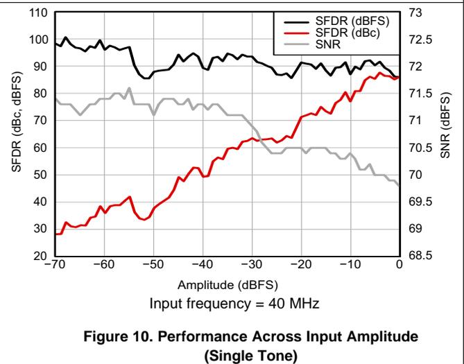
**Figure 10. Performance Across Input Amplitude (Single Tone)**
