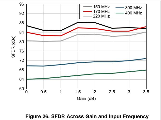
**Figure 26. SFDR Across Gain and Input Frequency**
