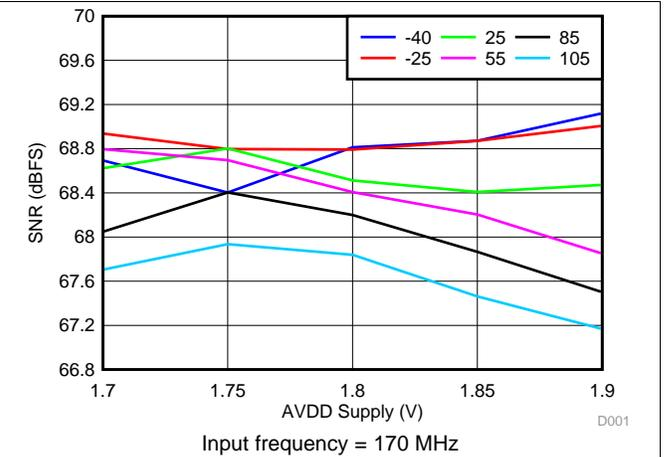
**Figure 14. SNR Across Ambient Temperature vs AVDD Supply**
