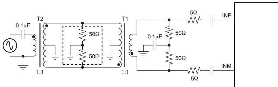
**Figure 86. Drive Circuit for High Input Frequencies**
