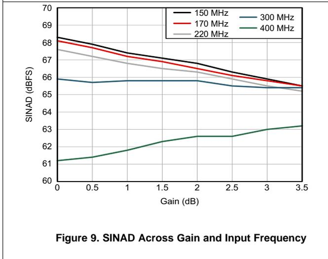
**Figure 9. SINAD Across Gain and Input Frequency**
