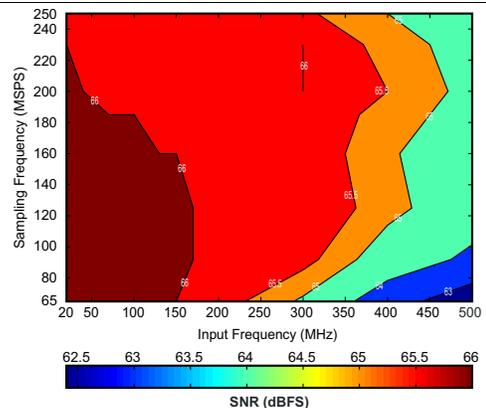
**Figure 47. SNR Contour (0-dB Gain, Applies to ADS41B29)**
