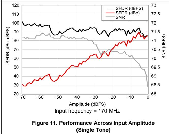
**Figure 11. Performance Across Input Amplitude (Single Tone)**
