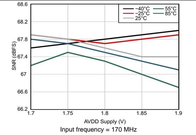
Figure 32. SNR Across Ambient Temperature vs AVDD Supply
