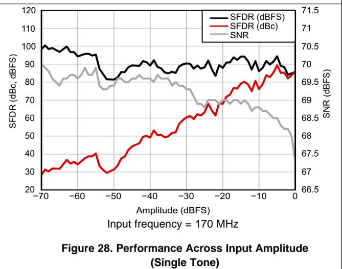
**Figure 28. Performance Across Input Amplitude (Single Tone)**
