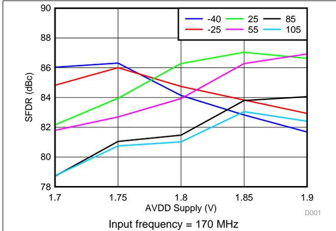
**Figure 13. SFDR Across Ambient Temperature vs AVDD Supply**
