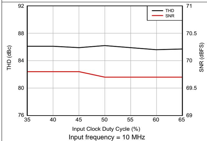
**Figure 17. Performance Across Input Clock Duty Cycle**
