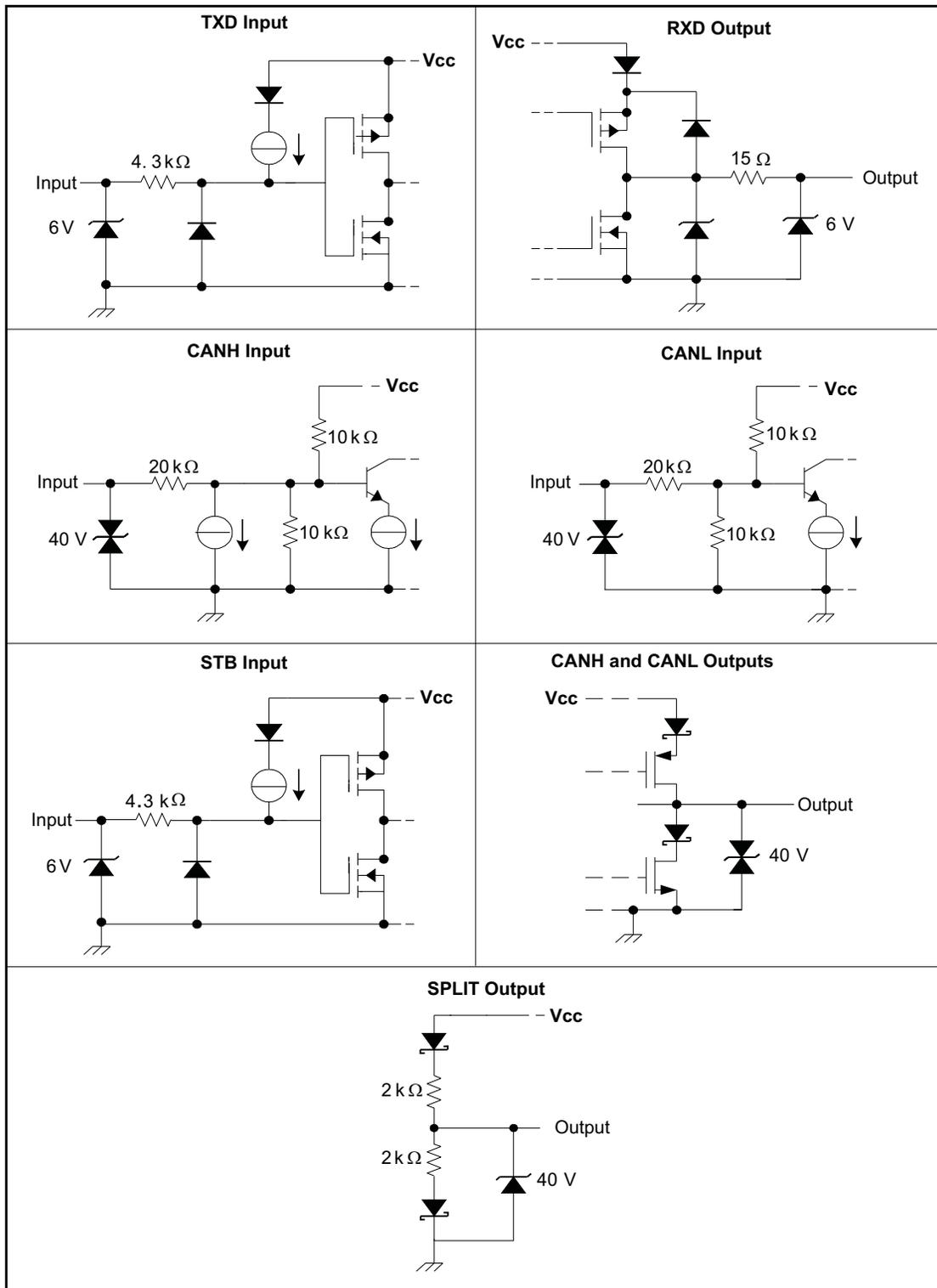
Figure 24. Equivalent Input and Output Schematic Diagrams
