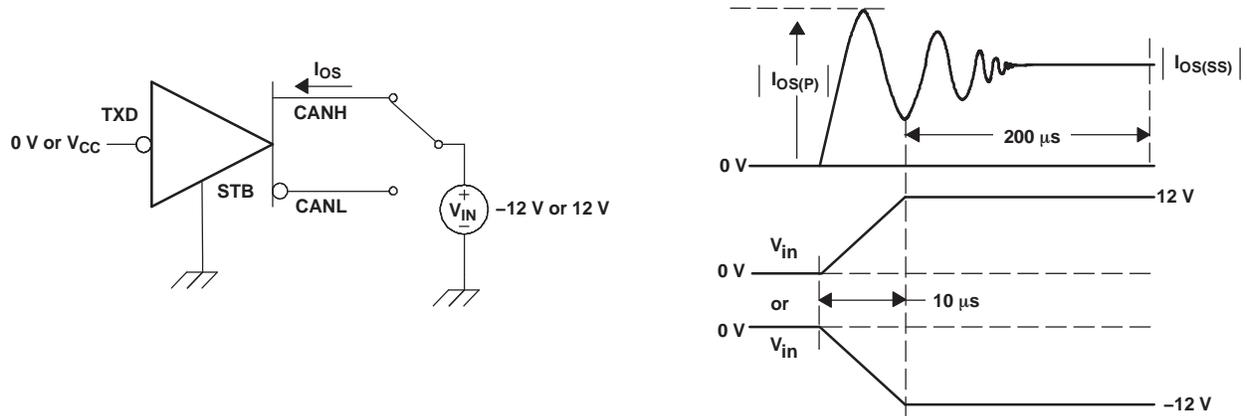
Figure 22. Driver Short-Circuit Current Test and Waveform
