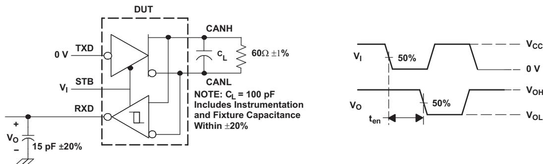
Figure 17.  $T_{en}$  Test Circuit and Voltage Waveforms
