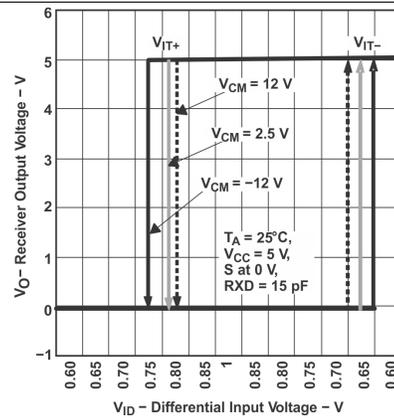
Figure 8. Receiver Output Voltage vs Differential Input Voltage
