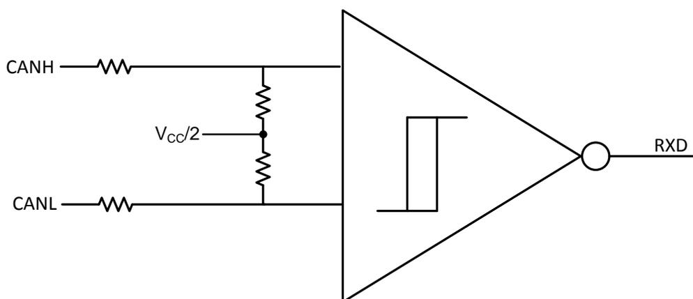
Figure 26. Simplified Recessive Common Mode Bias and Receiver
