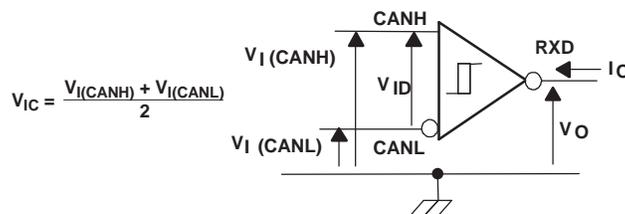
Figure 15. Receiver Voltage and Current Definitions
