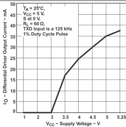
Figure 7. Driver Output Current vs Supply Voltage
