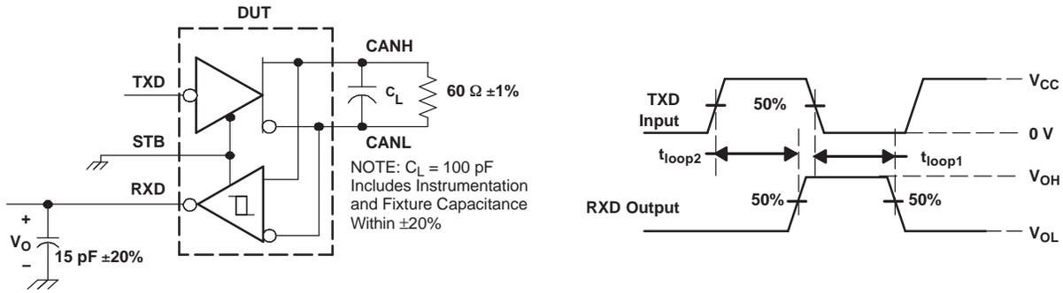
All  $V_I$  input pulses are from 0 V to  $V_{CC}$  and supplied by a generator with the following characteristics:  $t_r$  or  $t_f \leq 6 \text{ ns}$ . Pulse Repetition Rate (PRR) = 125 kHz, 50% duty cycle.
