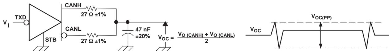
All  $V_I$  input pulses are from 0 V to  $V_{CC}$  and supplied by a generator having the following characteristics:  $t_r$  or  $t_f \leq 6$  ns. Pulse Repetition Rate (PRR) = 125 kHz, 50% duty cycle.
