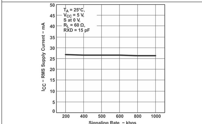
Figure 3. Supply Current (RMS) vs Signaling Rate
