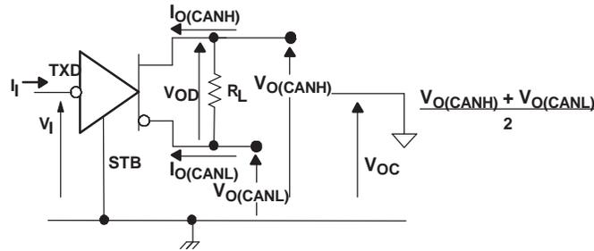
Figure 11. Driver Voltage, Current, and Test Definition
