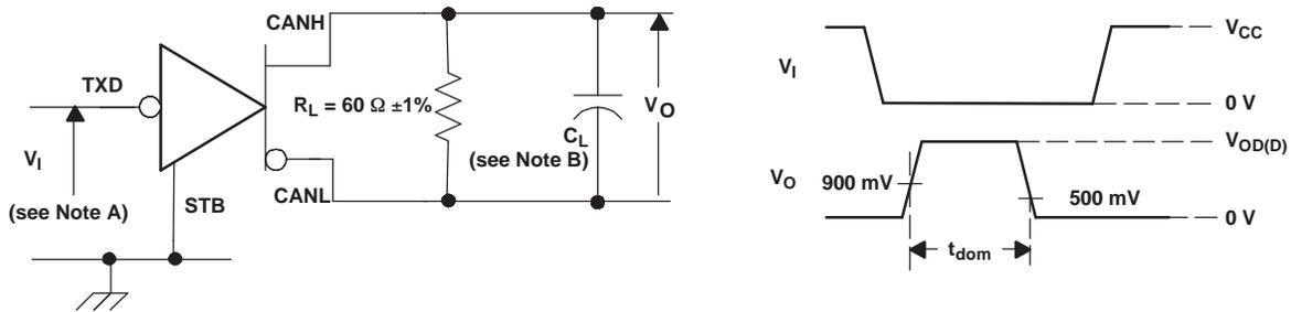
All  $V_I$  input pulses are from 0 V to  $V_{CC}$  and supplied by a generator with the following characteristics:  $t_r$  or  $t_f \leq 6 \text{ ns}$ . Pulse Repetition Rate (PRR) = 500 Hz, 50% duty cycle.
