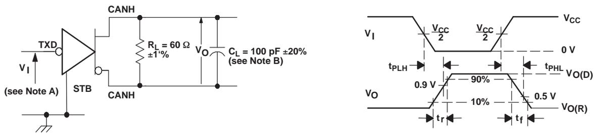
Figure 14. Driver Test Circuit and Voltage Waveforms
