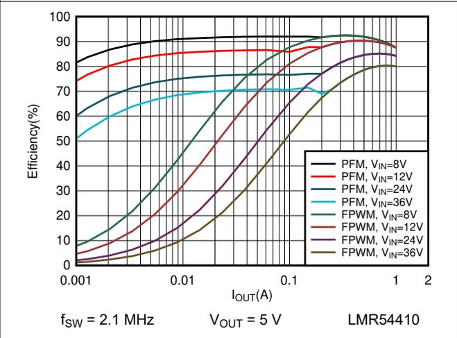
**Figure 7-4. 5-V Efficiency Versus Load Current**
