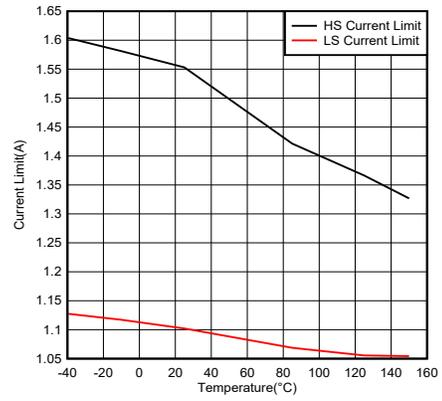
Figure 7-14. HS and LS Current Limit Versus Temperature
