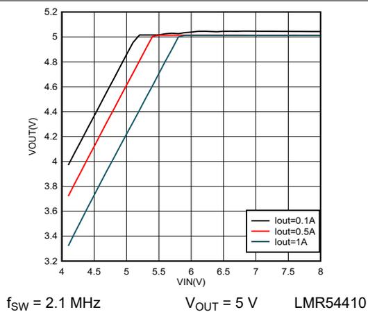
**Figure 7-9. 5-V Dropout**
