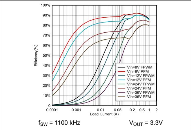
**Figure 7-2. 3.3-V Efficiency Versus Load Current - LMR54410**
