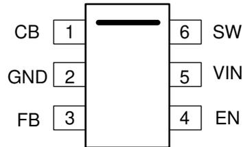
**Figure 6-1. 6-Pin SOT-23 DBV Package (Top View)**
