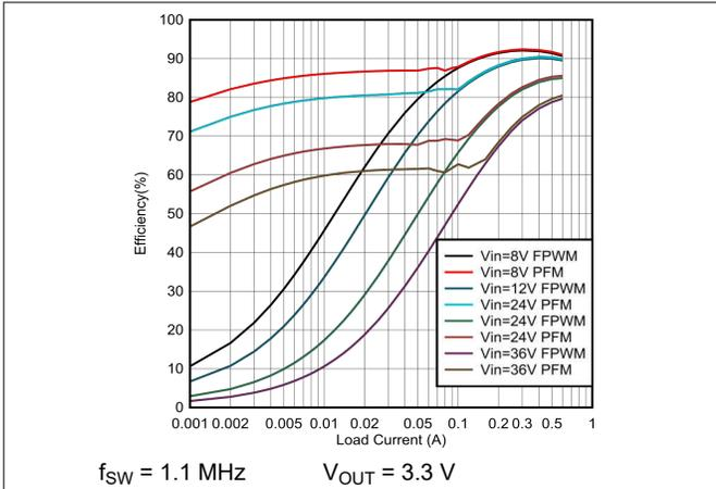
**Figure 7-1. 3.3-V Efficiency Versus Load Current - LMR54406**
