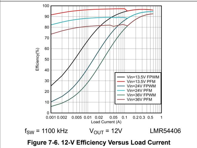
**Figure 7-6. 12-V Efficiency Versus Load Current**
