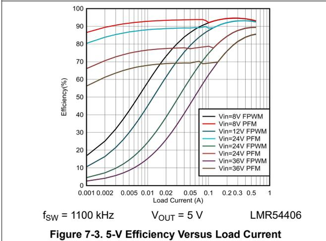
**Figure 7-3. 5-V Efficiency Versus Load Current**
