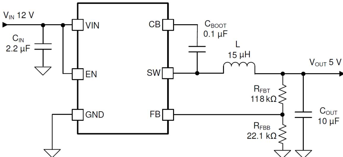
**Figure 9-1. Application Circuit**
