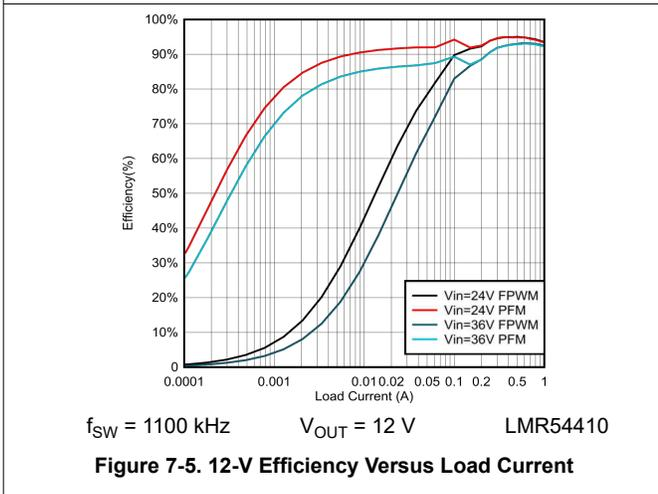
**Figure 7-5. 12-V Efficiency Versus Load Current**
