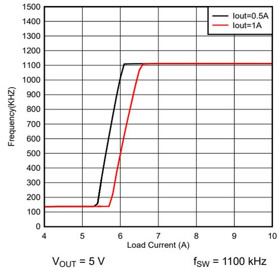
**Figure 8-5. Frequency Foldback at T<sub>OFF\_MIN</sub>**
