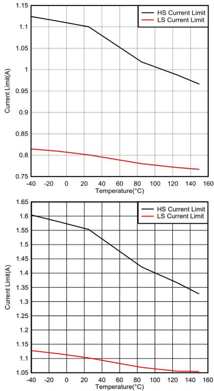
Figure 7-13. HS and LS Current Limit Versus Temperature
