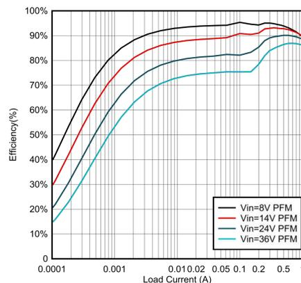
**Efficiency Versus Output Current;**
