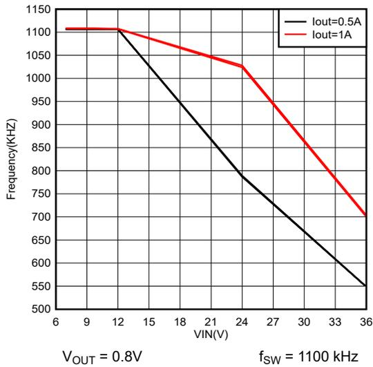
**Figure 8-4. Frequency Foldback at T<sub>ON\_MIN</sub>**
