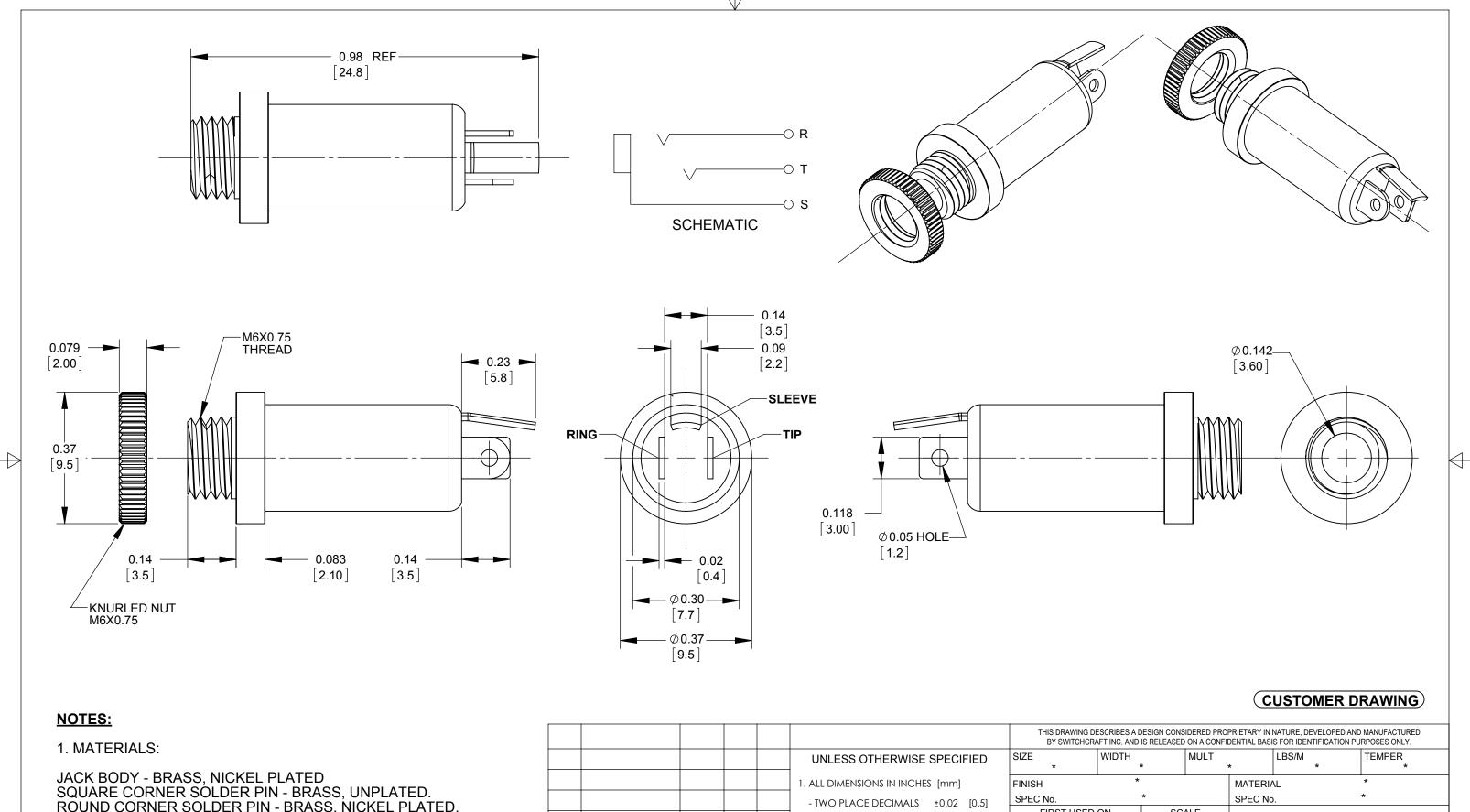
SQUARE CORNER SOLDER PIN - BRASS, UNPLATED. ROUND CORNER SOLDER PIN - BRASS, NICKEL PLATED. GROUND PIN - BRASS, NICKEL PLATED. NUT - BRASS, NICKEL PATED. INSULATOR - ABS, WHITE.
