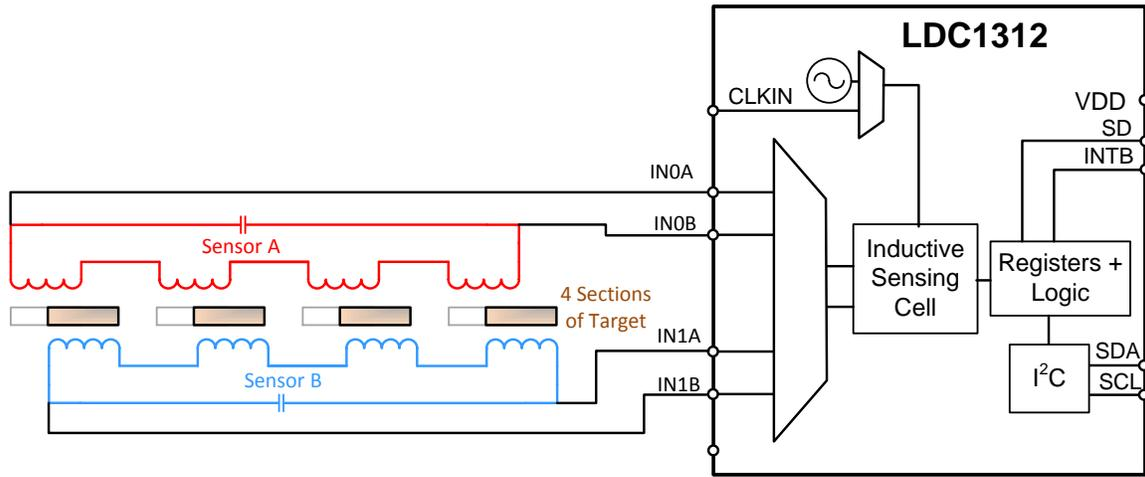
**Figure 17: Multiple Section Sensor Connection**
