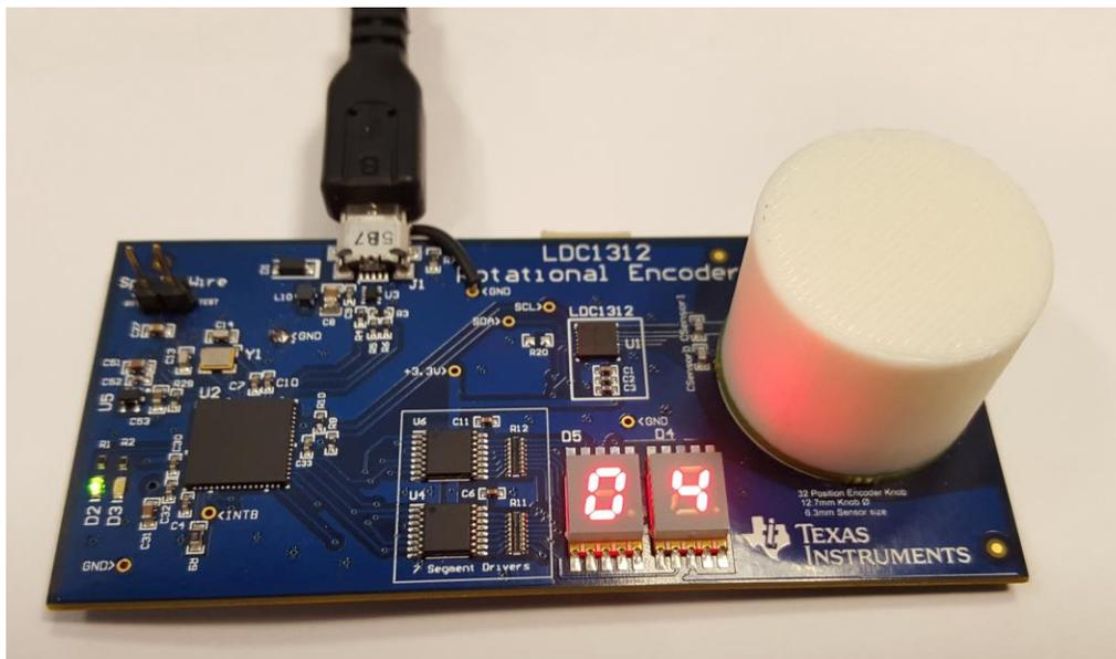
Figure 3: TIDA-00615 powered up by USB Connection after 4 steps
