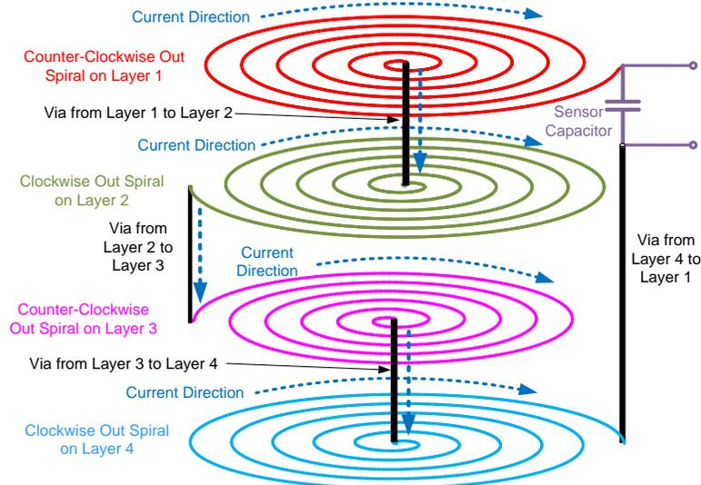
**Figure 16: 4-Layer Inductor physical construction**
