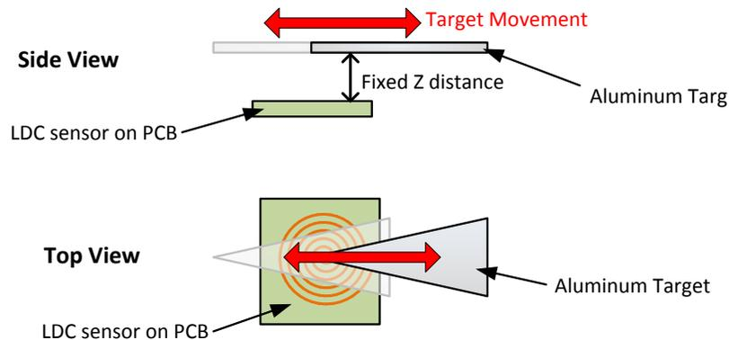
**Figure 10: Lateral Position Sensing with LDC**
