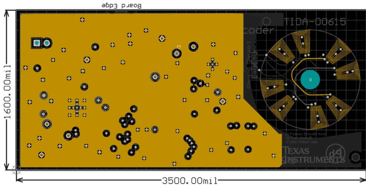
Figure 36: Sensor PCB Midlayer1 Routing
