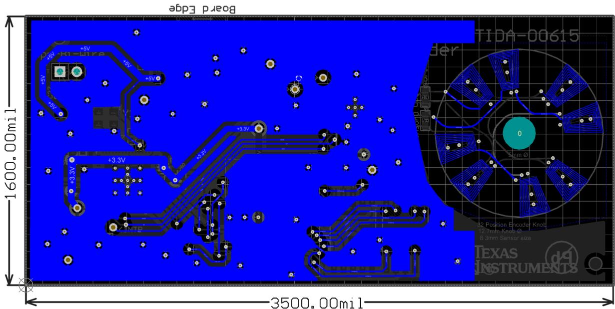
Figure 38: Sensor PCB Bottom Layer Routing
