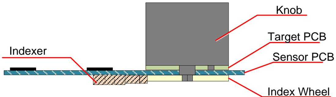
Figure 44: Mechanical Assembly
