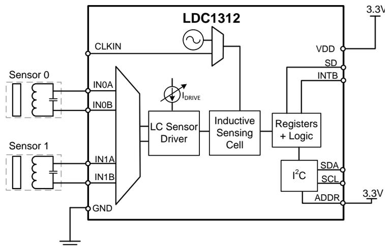
**Figure 11: LDC1312 Block Diagram**
