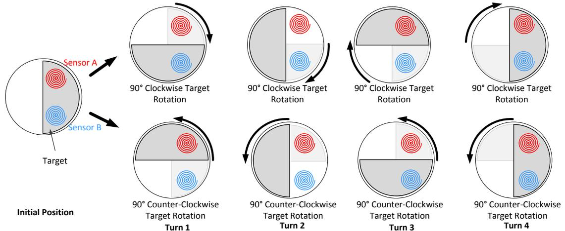
**Figure 12: Sensor and Target configuration**
