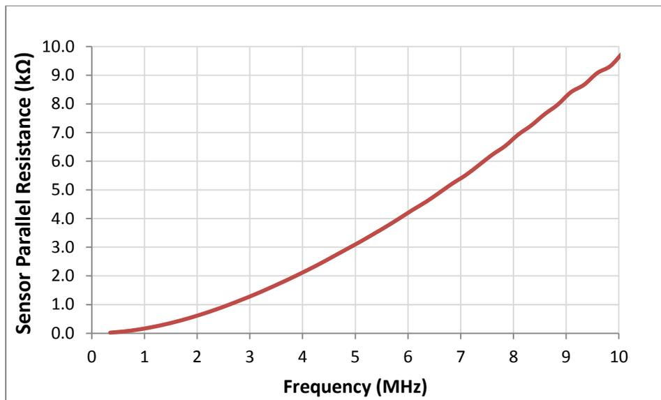
**Figure 21: Parallel Resistance [Ω] vs. Frequency sweep of each coil series**
