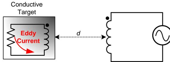
**Figure 4: Conductor in AC Magnetic Field**
