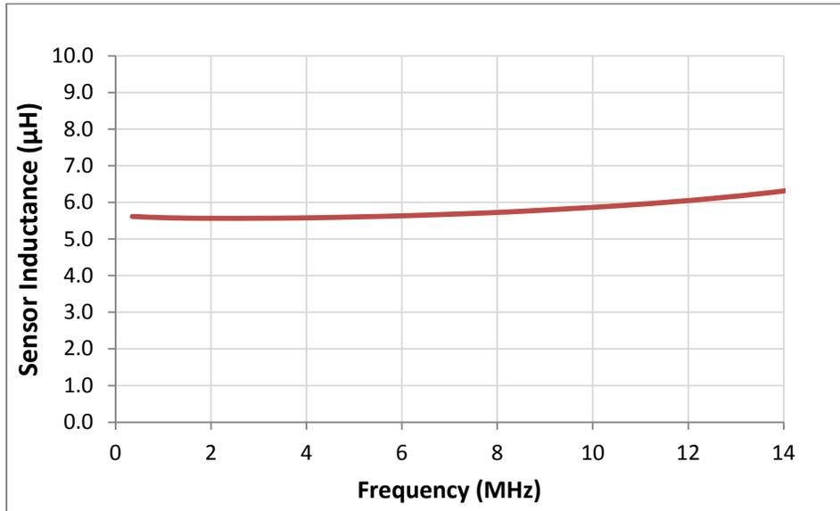
**Figure 20: Inductance (μH) vs. Frequency (MHz) of sensors**
