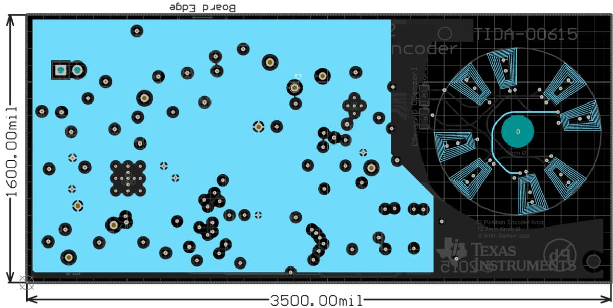
Figure 37: Sensor PCB Midlayer2 Routing
