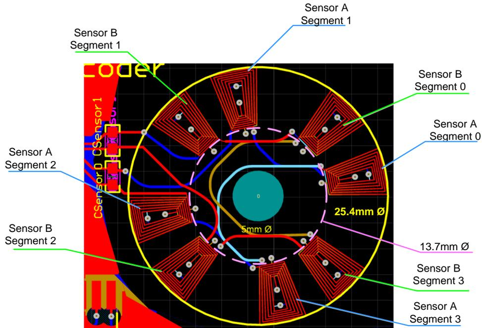
**Figure 18: Multiple Sensor Segment Geometry**
