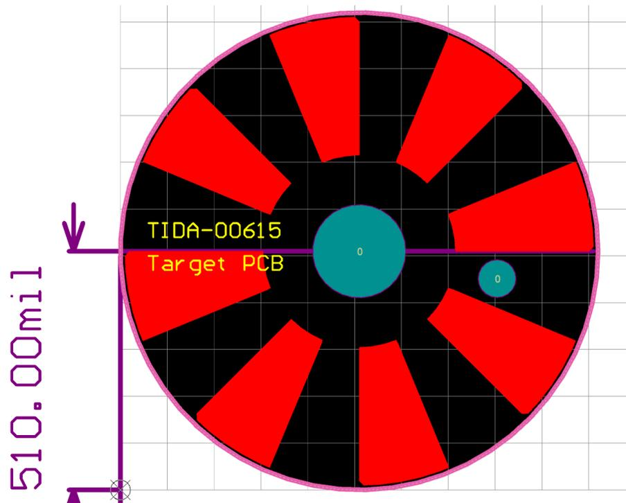
Figure 39: Target PCB Top Layer Routing
