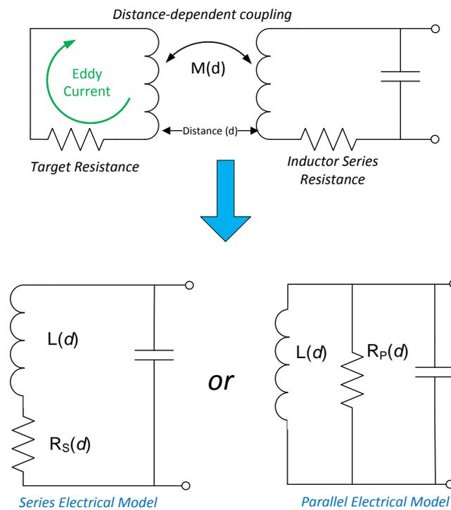
**Figure 5: Electrical Model of Parallel Inductive Sensor**
