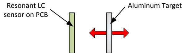
**Figure 6: Aluminum Target moved axially with respect to LC resonant circuit**
