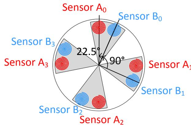
Figure 14: Equivalent Sensor placement for 16 position encoder
