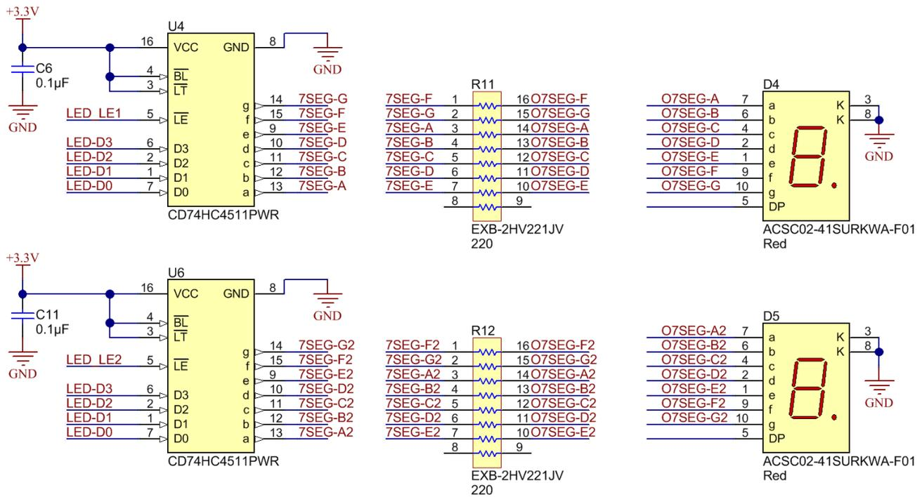
Figure 32: 7 Segment Displays and Drivers
