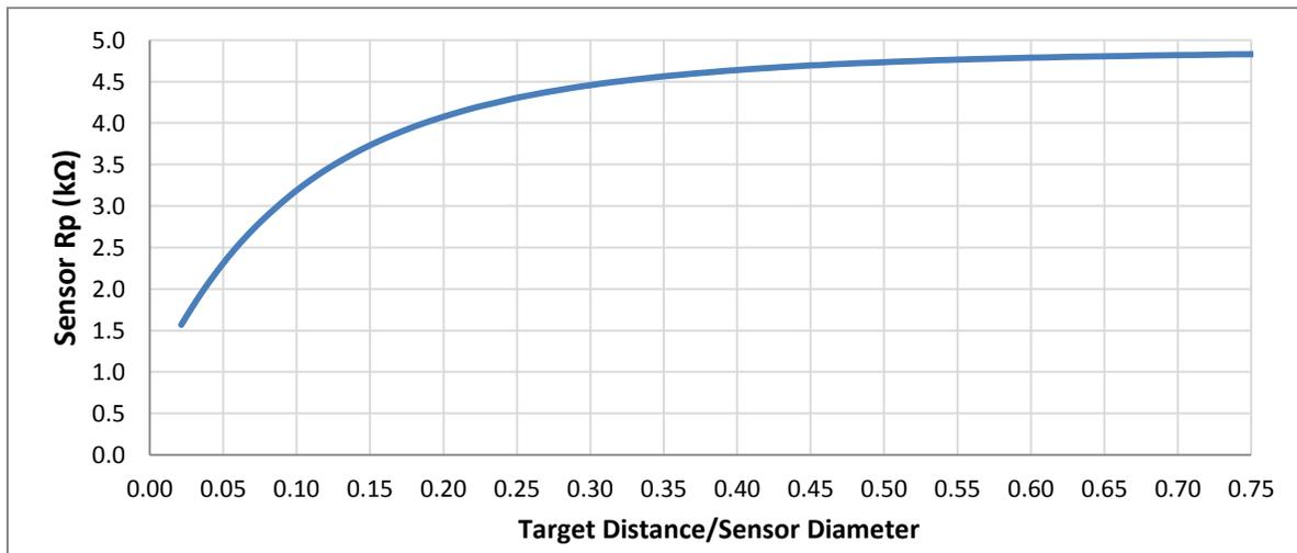
**Figure 9: Sensor  $R_p$  vs. Target Distance**
