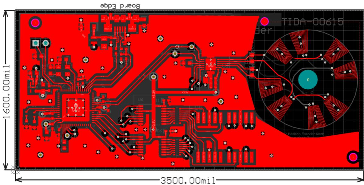
Figure 35: Sensor PCB Top Layer Routing
