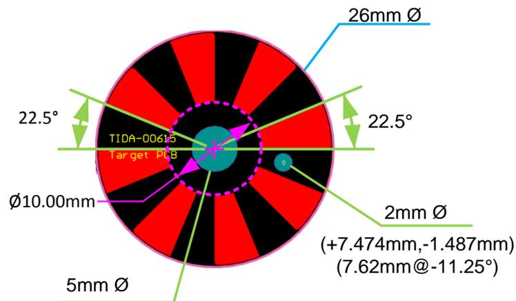
**Figure 19: Target Dimensions**
