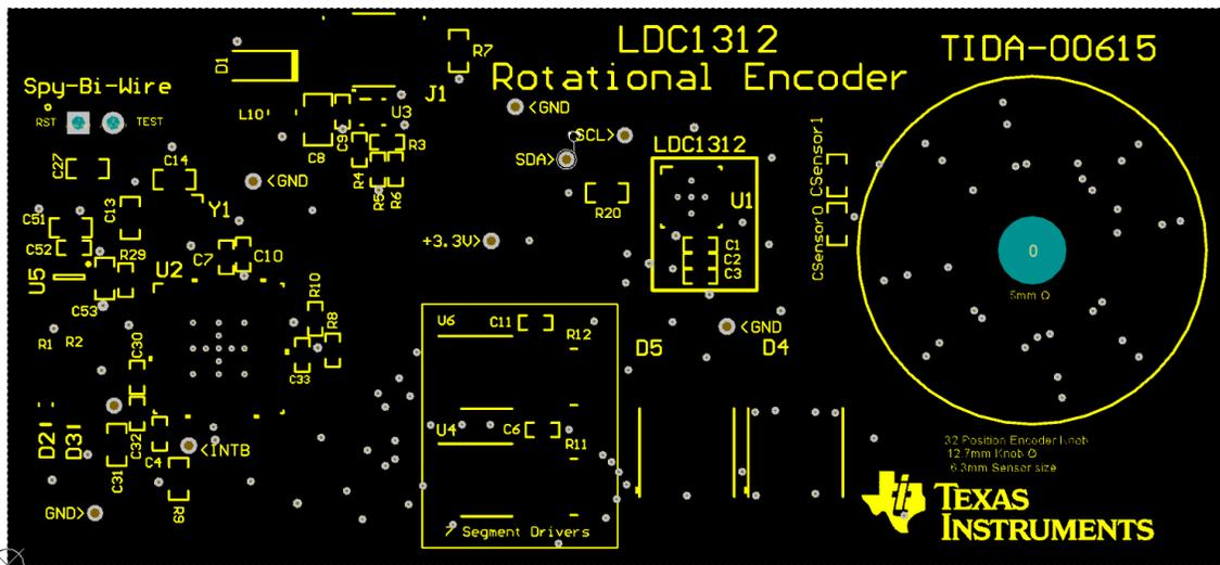
Figure 34: Sensor PCB Top Silkscreen
