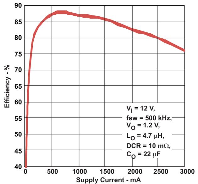
Figure 4. Buck 1 Efficiency,  $V_O = 1.2\text{ V}$ ,  $V_{IN} = 12\text{ V}$ ,  $f_{SW} = 500\text{ kHz}$ ,  $L_O = 4.7\text{ }\mu\text{H}$ ,  $\text{DCR} = 10\text{ m}\Omega$ ,  $C_O = 22\text{ }\mu\text{F}$
