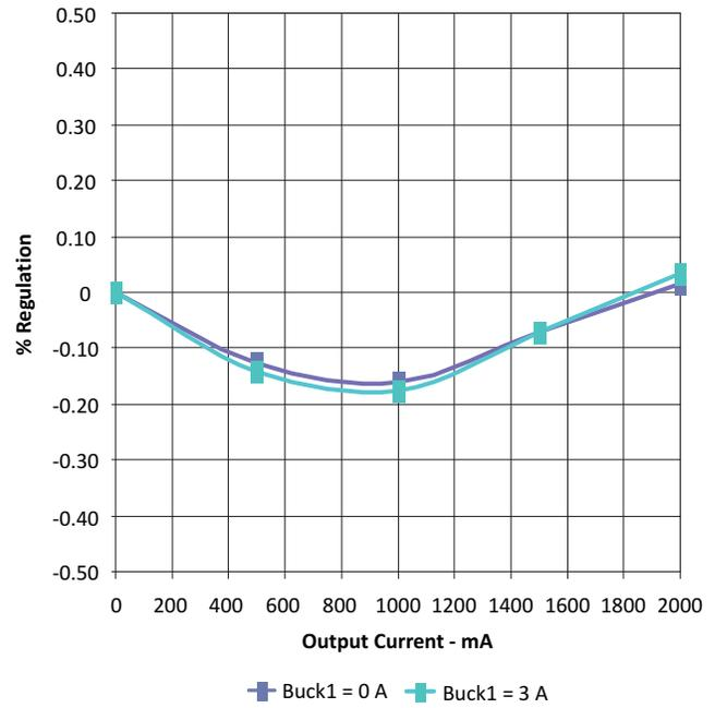
Figure 2. Buck2 Load Regulation  $V_O = 1.8\text{ V}$
