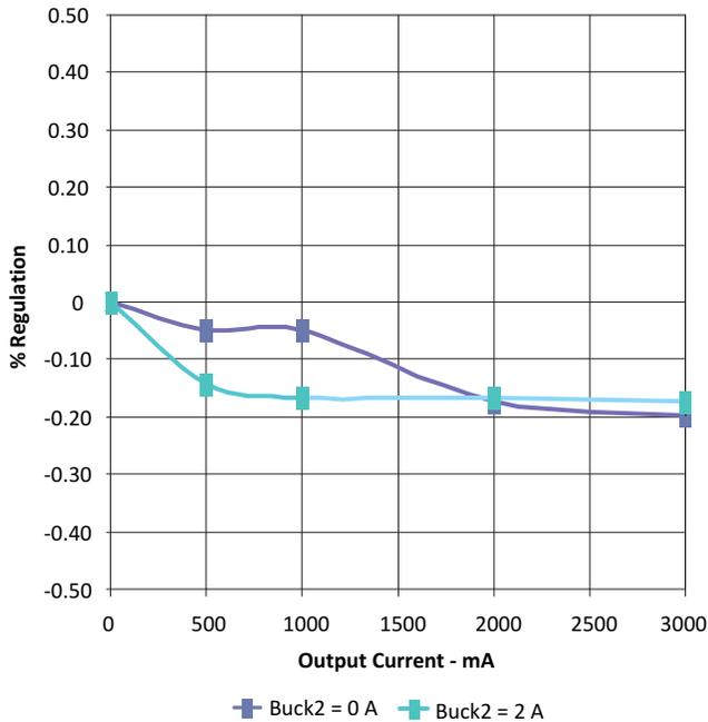
Figure 1. Buck1 Load Regulation,  $V_O = 1.2\text{ V}$
