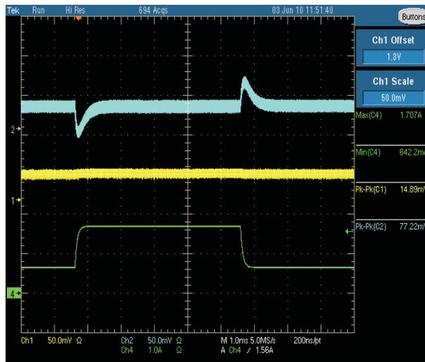
Figure 12. Buck 2 (Blue Trace) Dynamic Response 0.5-A - 1.5-A Step, 50 mV/div. Buck 1 (Yellow Trace), 50 mV/div
