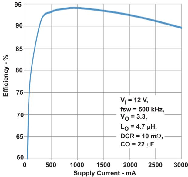
Figure 3. Buck 1 Efficiency,  $V_O = 3.3\text{ V}$ ,  $V_{IN} = 12\text{ V}$ ,  $f_{SW} = 500\text{ kHz}$ ,  $L_O = 4.7\text{ }\mu\text{H}$ ,  $\text{DCR} = 10\text{ m}\Omega$ ,  $C_O = 22\text{ }\mu\text{F}$
