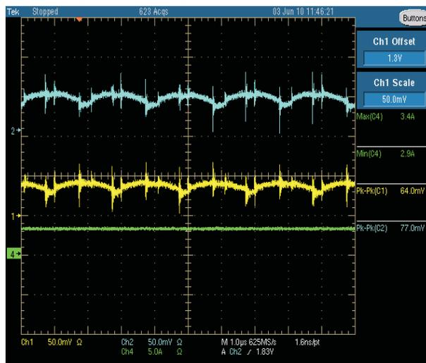
Figure 10. Ripple for Buck 1 (Yellow Trace) 1.2 V, 3 A and Buck 2 (Blue Trace) 1.8 V, 2 A, 50 mV per Division
