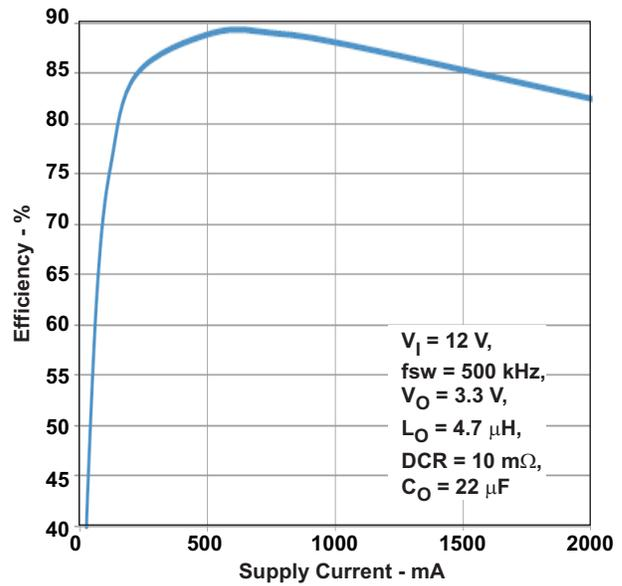
Figure 6. Buck 2 Efficiency,  $V_O = 3.3\text{ V,}$
