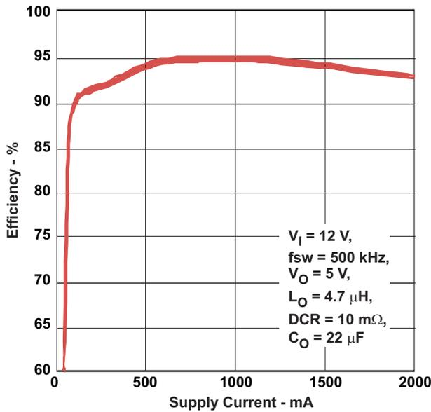
Figure 5. Buck 2 Efficiency,  $V_O = 5\text{ V,}$
