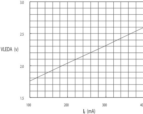
Figure 4. **I<sub>F</sub>-LEDA Characteristics (0°)**
