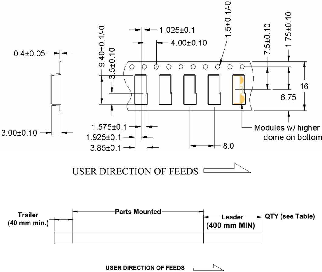
Figure 10. ZHX1810 Tape Dimensions and Configuration (Unit: mm)
