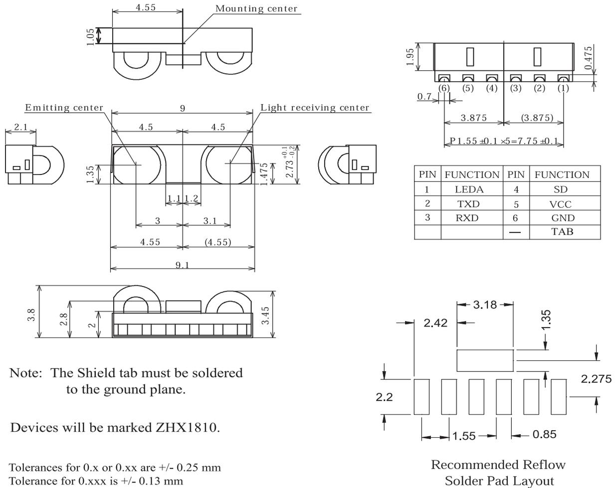
Note: The Shield tab must be soldered to the ground plane.
