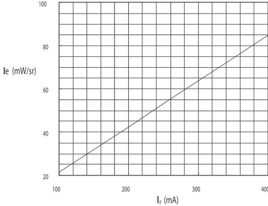
Figure 3. **I<sub>F</sub>-I<sub>e</sub> Characteristics (0°)**
