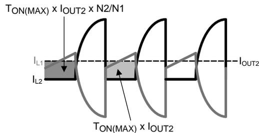
Figure 13. Current Waveforms for  $C_{OUT1}$  Ripple Calculation
