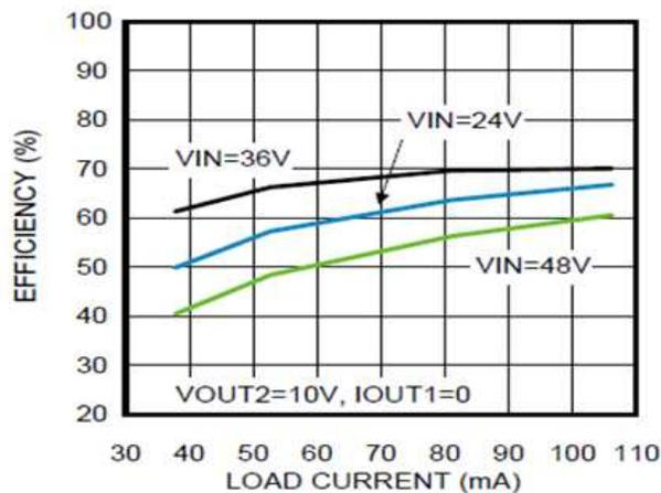
Figure 16. Efficiency at 750 kHz,  $V_{OUT1} = 10 \text{ V}$
