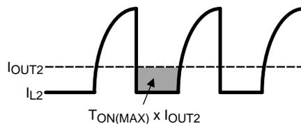
Figure 14. Secondary Current Waveforms for  $C_{OUT2}$  Ripple Calculation
